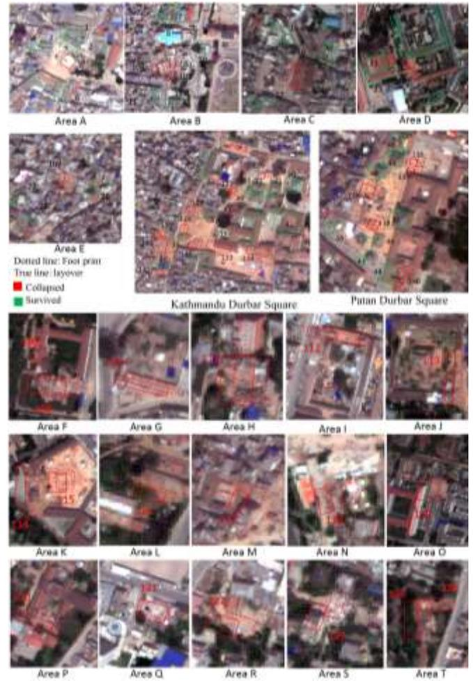
**Fig.4.** Training area in the central Kathmandu: 41 Collapsed • Major damaged buildings and 50 No • Minor damaged buildings with rooftop and layover of each building
