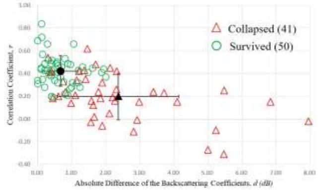
**Fig. 5.** Scatter diagram of correlation coefficient and difference of backscattering coefficient of the collapsed building and survived building
