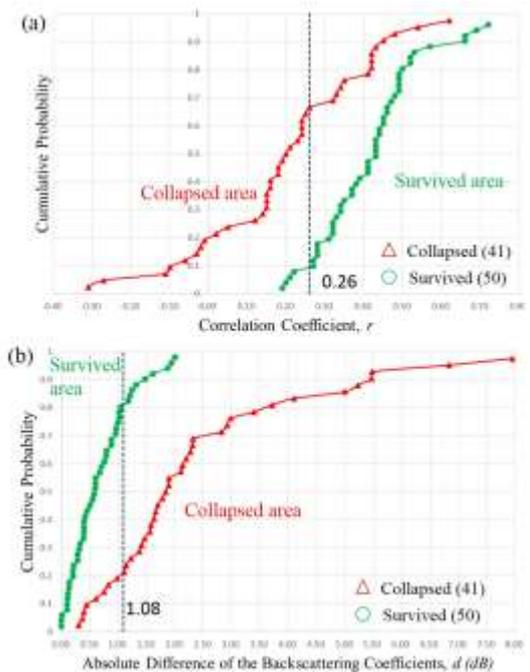
**Fig. 6.** Cumulative probability of the (a) correlation coefficient and (b) difference value of the 41 collapsed buildings and 50 survived building
