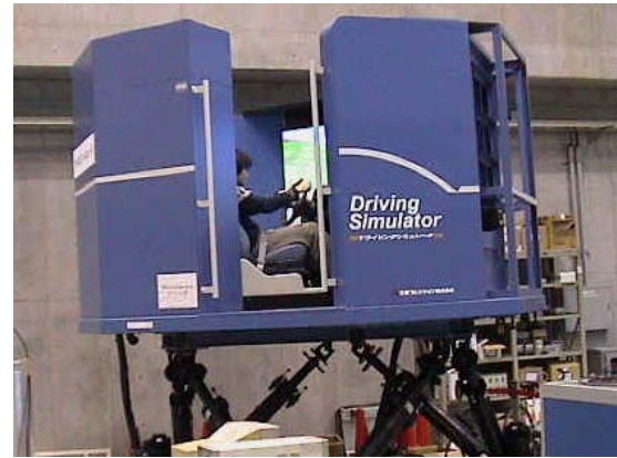
Fig. 4. Driving simulator installed to Institute of Industrial Science, the University of Tokyo
