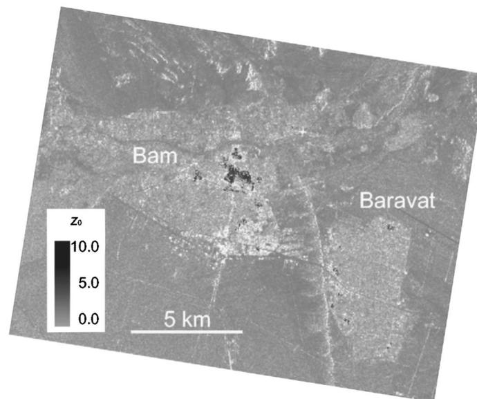
**Figure 3.** Distribution of the  $z_0$  value, which is derived from a damage detection method (Matsuoka and Yamazaki 2004), using Envisat images taken before (03 December 2003) and after (07 January 2004) the 2003 Bam, Iran earthquake.
