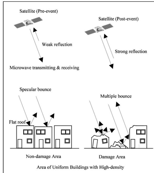
**Figure 8.** Schematic figure of the backscattering characteristics of orderly uniform buildings with flat roofs and their damages.
