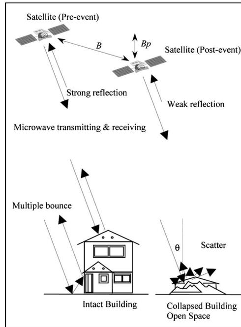
**Figure 1.** Schematic figure of the repeat pass satellite observation geometry and backscattering characteristics of buildings.
