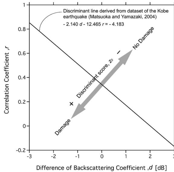
**Figure 2.** Schematic figure for estimating the severely damaged area using two indices, the difference in the backscattering coefficient and the correlation coefficient calculated from pre- and post-earthquake SAR intensity images.
