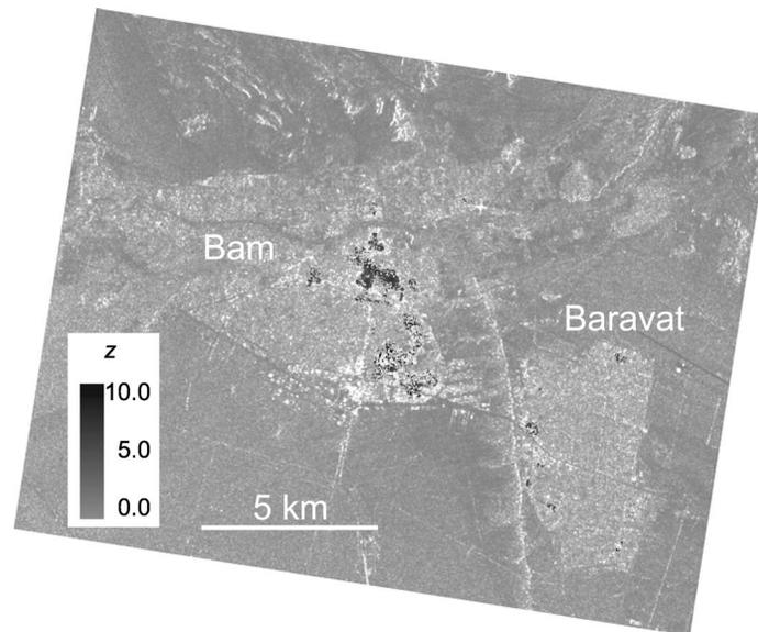
**Figure 10.** Distribution of the  $z$  value, which is derived from a revised method using the pair of Envisat images.
