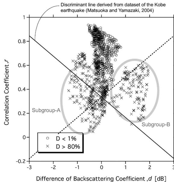
**Figure 9.** Difference in the backscattering coefficient and correlation coefficient of a less damaged area where the ratio of Grade 5 damaged buildings ( $D$ ) is less than 1%, and a severely damage area where the  $D$  is more than 80%. The solid line indicates the discriminant line from the data set of the 1995 Kobe earthquake (Matsuoka and Yamazaki 2004). The dotted line is another line that is assumed to distinguish the less damaged area and Subgroup B in the severely damage areas.
