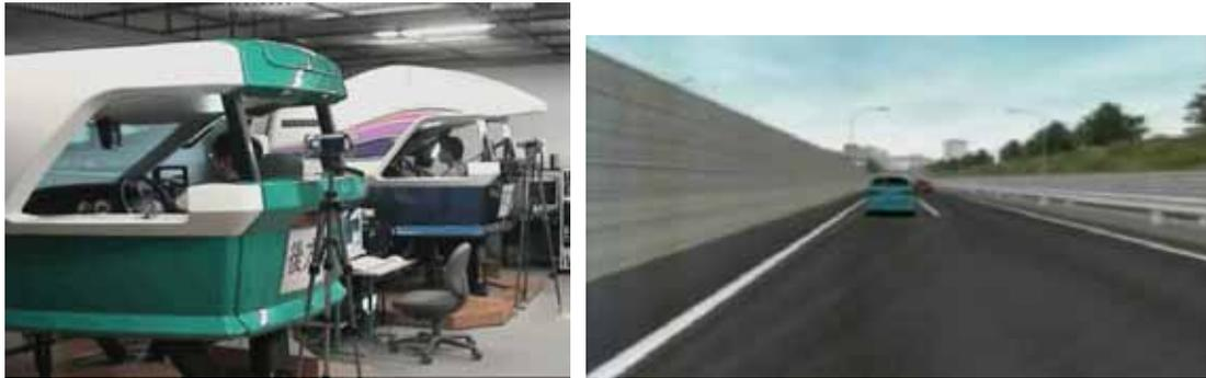
Fig. 8. Two regular driving simulators used in the experiment and the front view from the rear vehicle.
