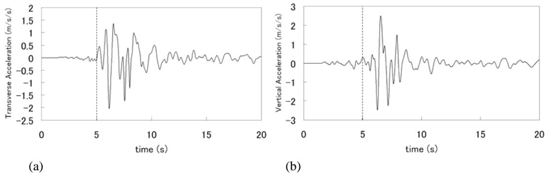
Fig. 3. Response acceleration time histories to (a) the transverse direction and (b) vertical direction of the moving vehicle under the JR Takarazuka record when the vehicle is moving at the speed of 120 km/h.
