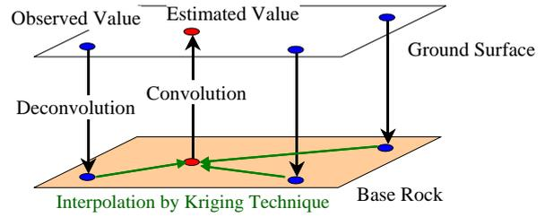
**Fig.1** Schematic figure for interpolation of strong motion indices.
