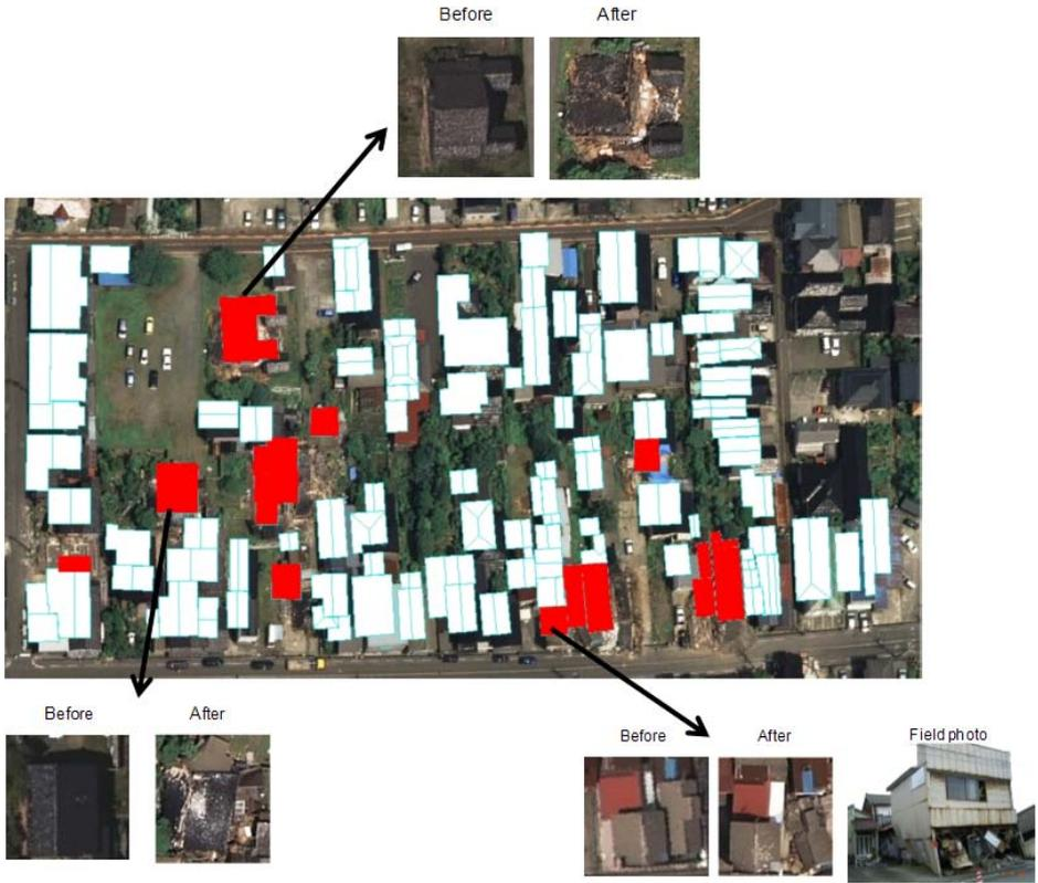
Fig. 8. (Color online) Examples of visual damage inspection using aerial images and field photos and detected collapsed buildings by this study.
