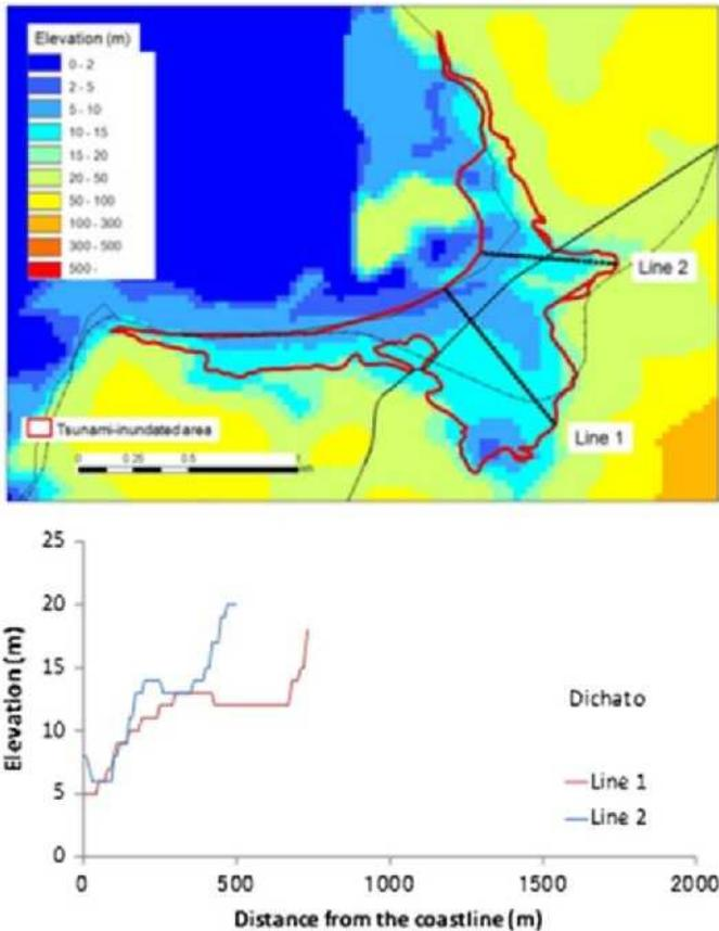
**Figure 7.** Tsunami-inundated areas and distribution of the elevations in Dichato and elevations along the transverse lines.
