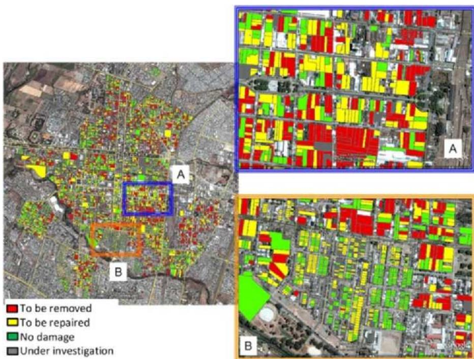
**Figure 2.** GIS file to show the damage levels of buildings in Talca.
