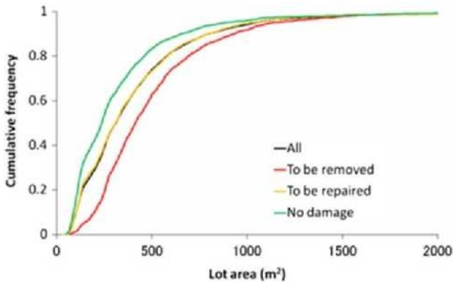
**Figure 3.** Cumulative frequencies of the areas of building lots with respect to the damage level. The red rectangles indicate the affected areas that were detected visually.
