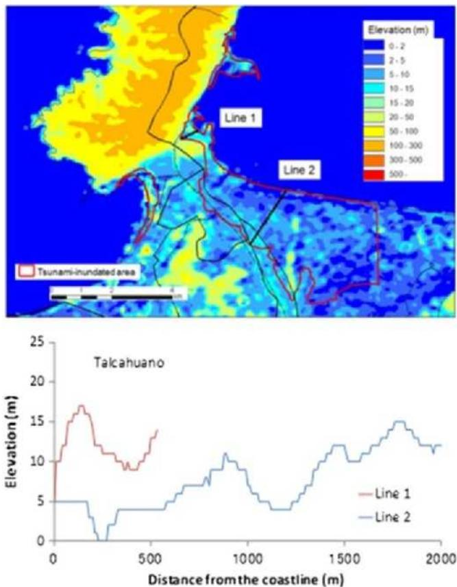
**Figure 6.** Tsunami-inundated areas and distribution of the elevations in Talcahuano and elevations along the transverse lines.
