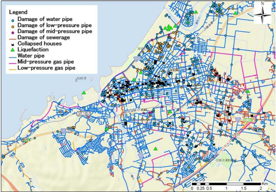
Fig. 1. Inventory data and damage data of lifeline systems in Kashiwazaki city due to the 2007 Niigata Chuetsu-Oki earthquake.
