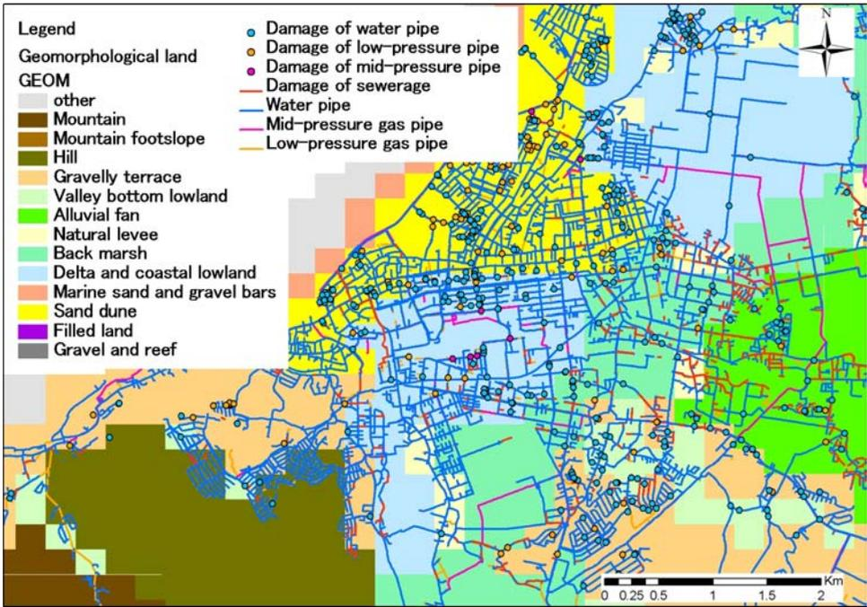
Fig. 2. Damage incidents to buried pipes in Kashiwazaki city after the 2007 Niigata Chuetsu-Oki earthquake illustrated on the geomorphological land classification map by Wakamatsu *et al.* [2006].
