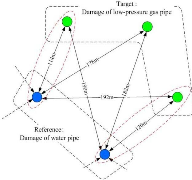
Fig. 6. Definition of the shortest distances between damage incidents.
