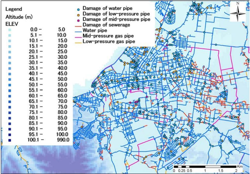
Fig. 4. Spatial distributions of altitude and damage incidents to buried pipes in Kashiwazaki city after the 2007 Niigata Chuetsu-Oki earthquake.
