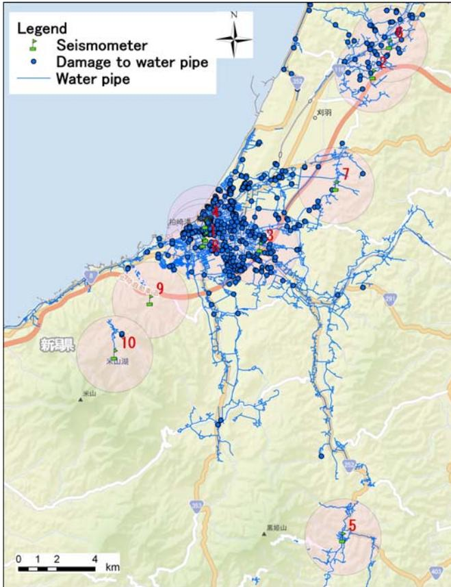
Fig. 7. Location of seismometers in Kashiwazaki city and damage incidents to water distribution pipe after the 2007 Niigata Chuetsu-Oki earthquake.
