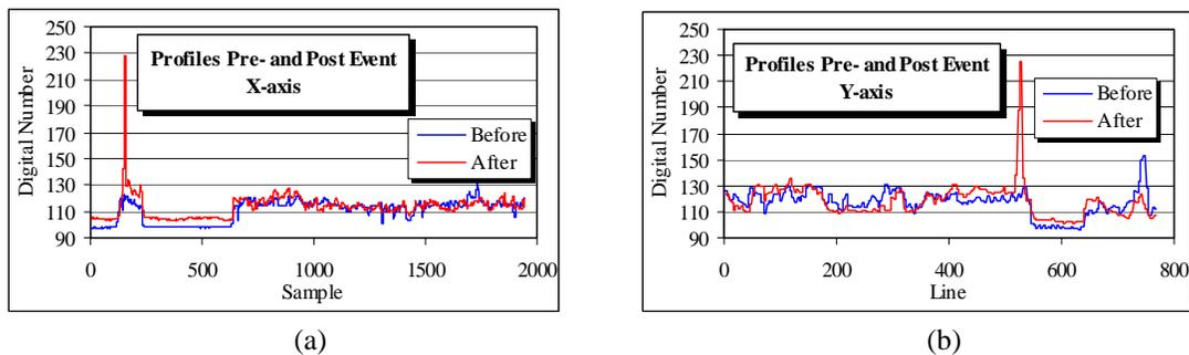
**Figure 3.** Profiles of the pre- and post-event images of the band 6. (a) Profile along the X-axis. (b) Profile along the Y-axis. Notice the peak value that represent the area around Tüpras refinery.
