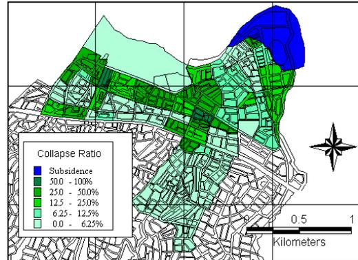
**Figure 9.** Distribution of the damage in Gölcük (AIJ, 1999).
