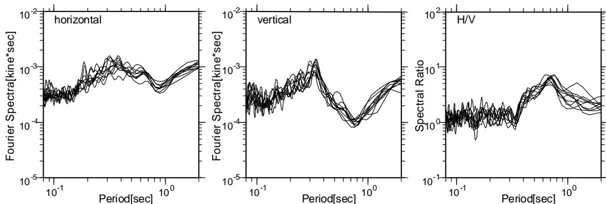
Figure 3. Horizontal and vertical Fourier spectra, and H/V Fourier spectral ratios of microtremor at K-NET Miyazaki station in Miyazaki City.
