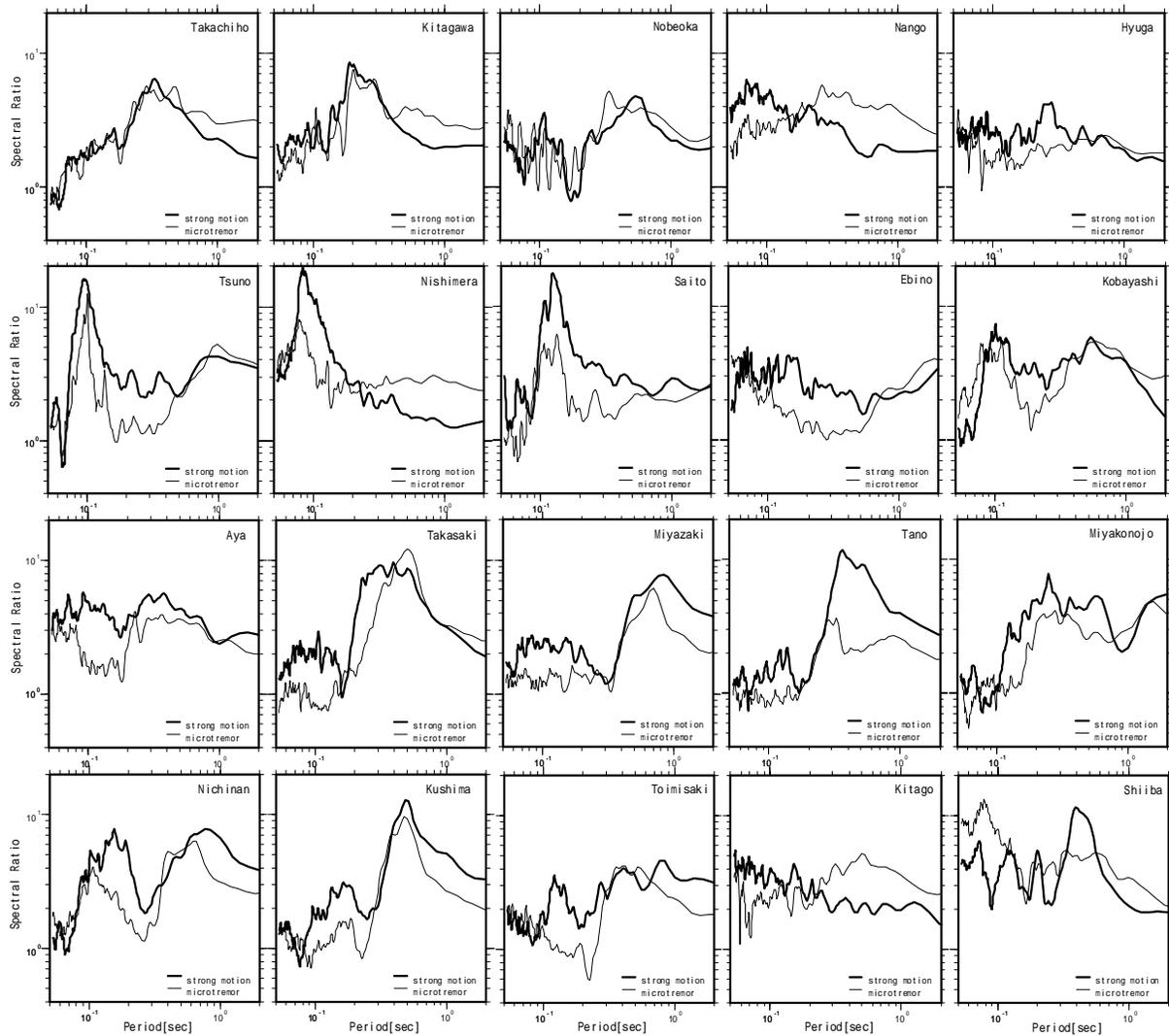
Figure 4. Comparison of the H/V Fourier spectral ratios for strong motion and microtremor.
