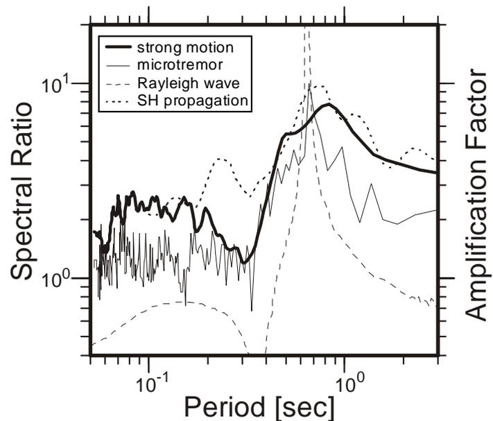
Figure 5. Comparison of the H/V Fourier spectral ratios of strong motion and microtremor, H/V amplitude ratio Rayleigh wave and the transfer function for S-wave propagation for K-NET Miyazaki station.
