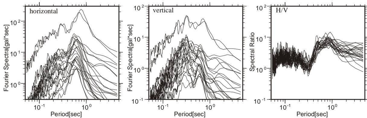
Figure 2. Horizontal and vertical Fourier spectra, and H/V Fourier spectral ratios of seismic ground motion at K-NET Miyazaki station in Miyazaki City.
