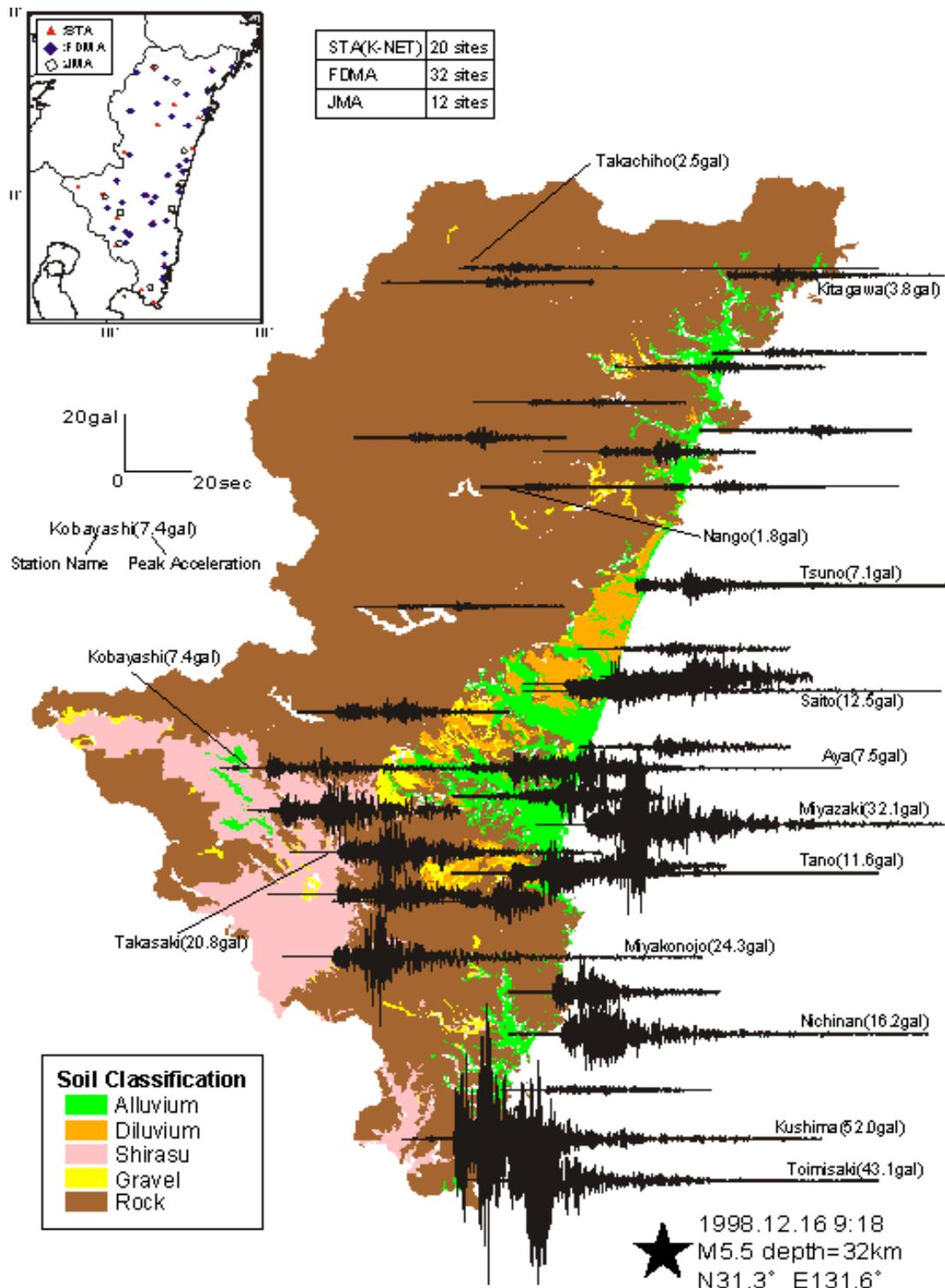
Figure 1. Distribution of seismometers in Miyazaki prefecture and seismic records in a magnitude 5.5 earthquake.
