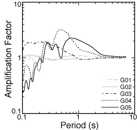
Figure 7. Amplification factors between Sites G01-G05 and the bedrock for vertically incident S-waves.
