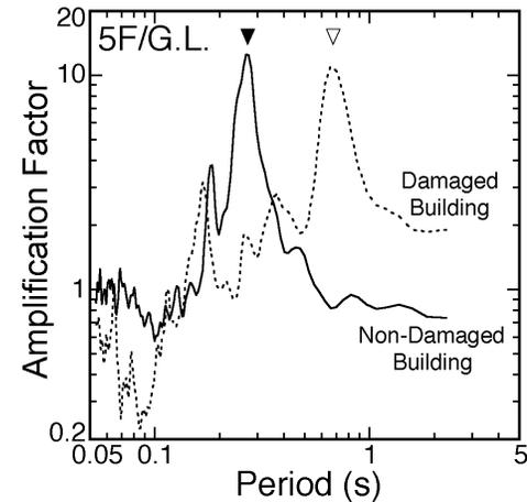
Figure 8. Amplification factors between the top and ground floors of the damaged and non-damaged buildings.
