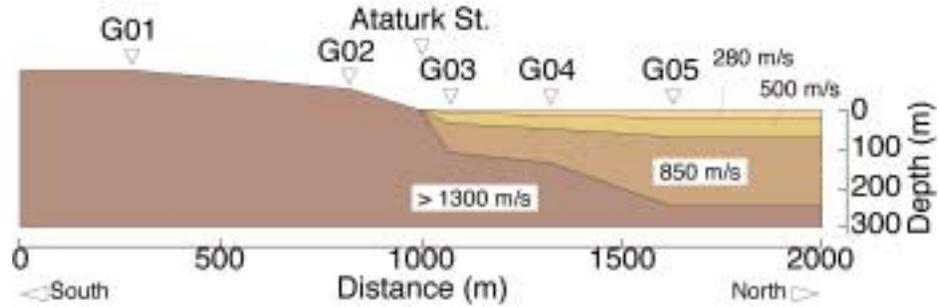
Figure 4. Estimated two-dimensional  $V_s$  profile along the line passing through Sites G01-G05.
