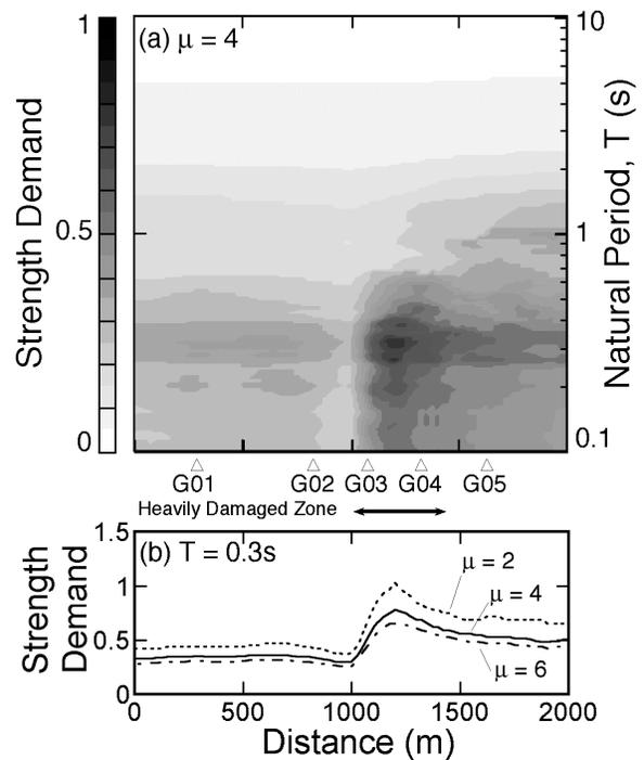
Figure 9. Variation of strength demand spectra computed for the simplified SDOF building systems along the observation line.
