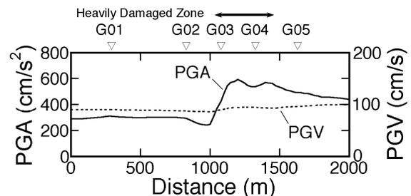
Figure 5. Variation of PGA and PGV of the simulated motions along the observation line.
