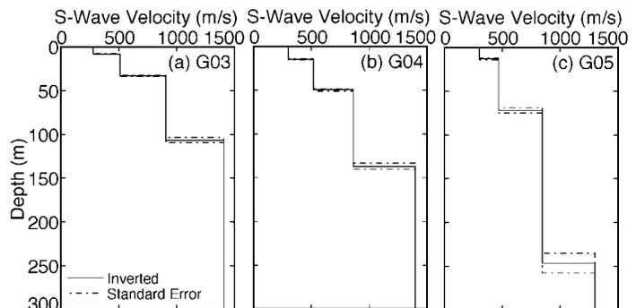
Figure 3. Inverted  $V_S$  profiles with standard errors of layer thickness at Sites G03-G05.
