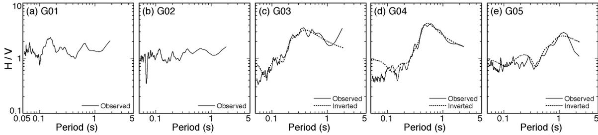
Figure 2. H/V spectra of microtremors compared with those of Rayleigh waves theoretically computed for the inverted soil layer models at Sites G01-G05.
