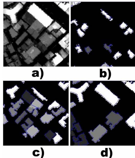
Figure 3. Extracted building polygons overlaid on raster images: a) original DHM image, b), c) and d) extracted building features from fine to coarse scales.
