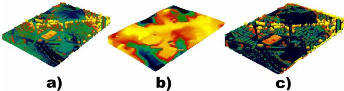
Figure 1. Results of LiDAR point classification a) DSM, b) DTM, and c) DHM.
