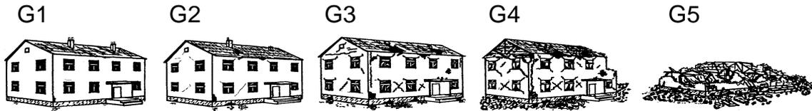
Fig. 4 Classification of damage to masonry buildings (EMS 1998)
