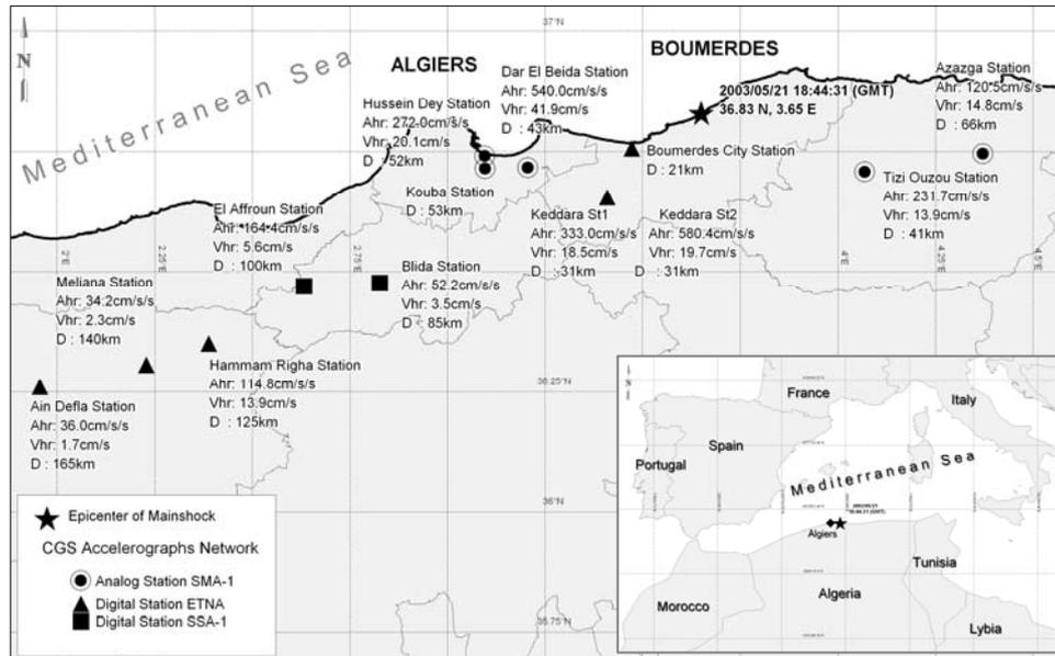
Figure 1 Location of the location (star) of the 2003 Boumerdes earthquake and the CGS accelerograph network that recorded the mainshock. Ahr and Vhr are the maximum resultants of the horizontal acceleration and velocity, respectively. D is the hypocentral distance.
