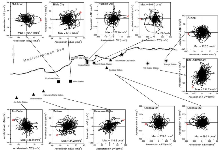
Figure 4 Particle traces of the acceleration records at different seismic stations. Open circle corresponds to the direction of the maximum resultant value.
