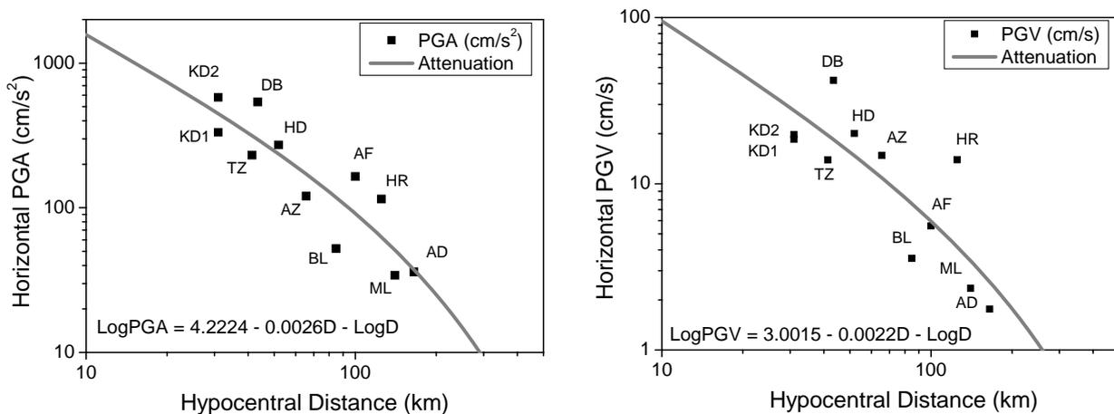
Figure 3 Attenuation law of seismic motion in terms of PGA and PGV
