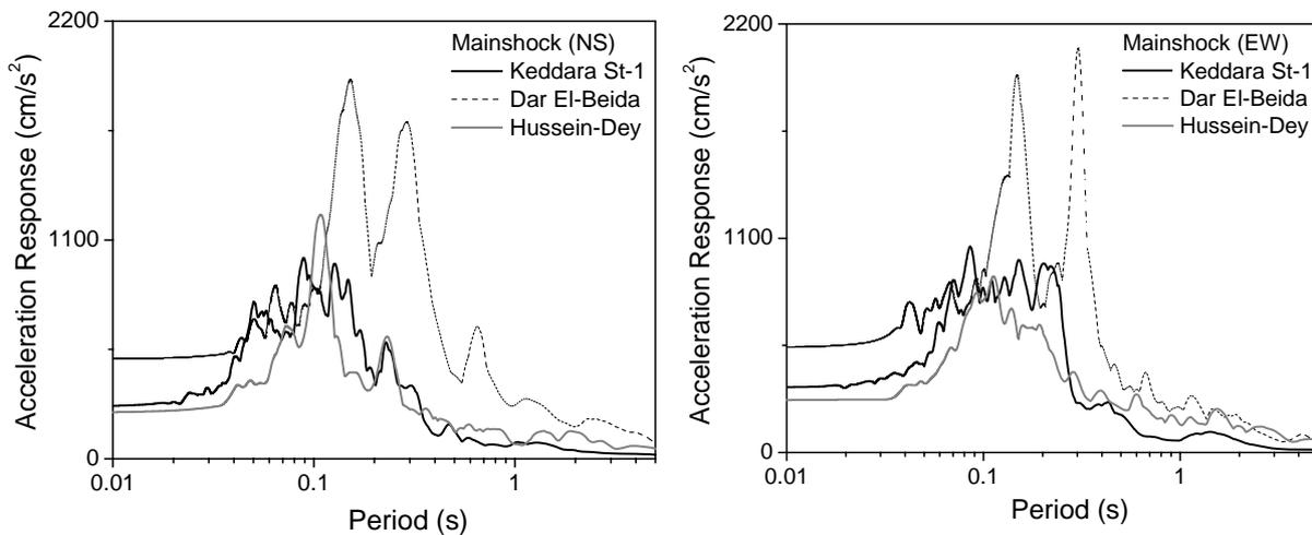
Figure 7 Acceleration response spectra of recorded mainshock at Keddara, Dar El-Beida and Hussein-Dey.
