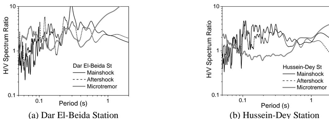
Figure 10 Comparison of H/V spectral ratios between microtremor and seismic motions at Dar El-Beida and Hussein-Dey.
