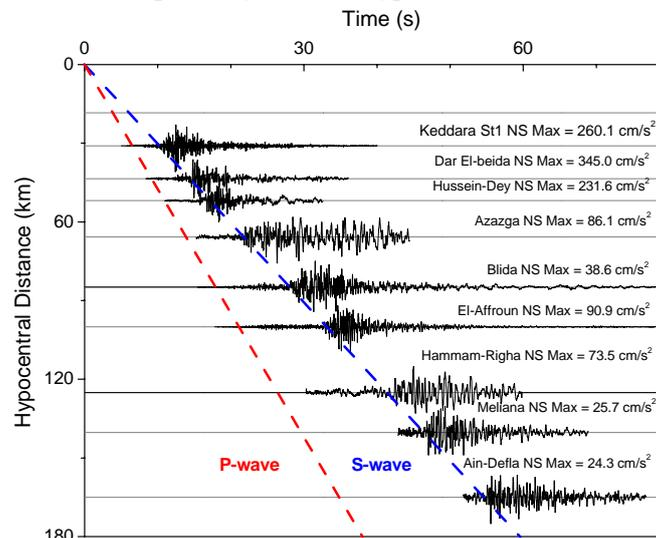
Figure 2 The estimated starting time of the mainshock and seismic wave propagation in the 2003 Boumerdes, Algeria earthquake (NS components).
