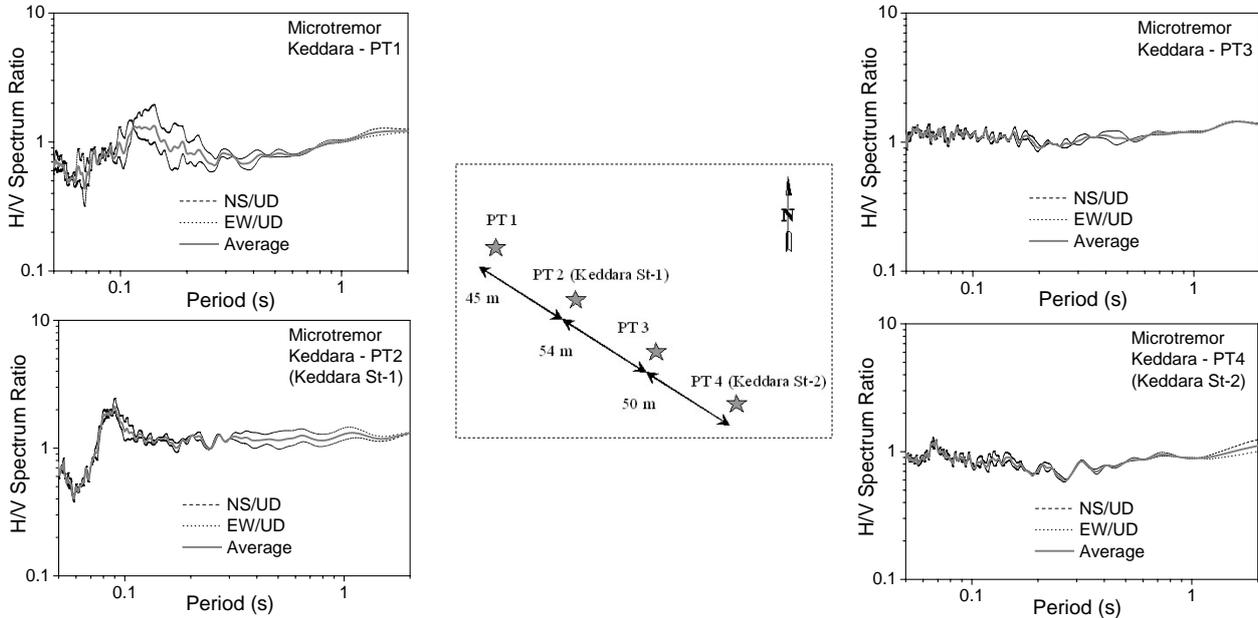
Figure 8 Layout of microtremor measurement points and H/V ratio in Keddara. PT2 and PT4 correspond to Keddara seismic stations 1 and 2, respectively. PT1 and PT3 are the added points for microtremor
