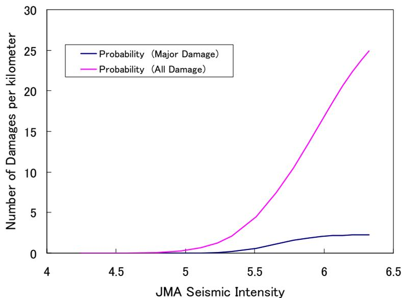
Figure 9 Fragility curves of expressway embankment with respect to JMA seismic intensity
