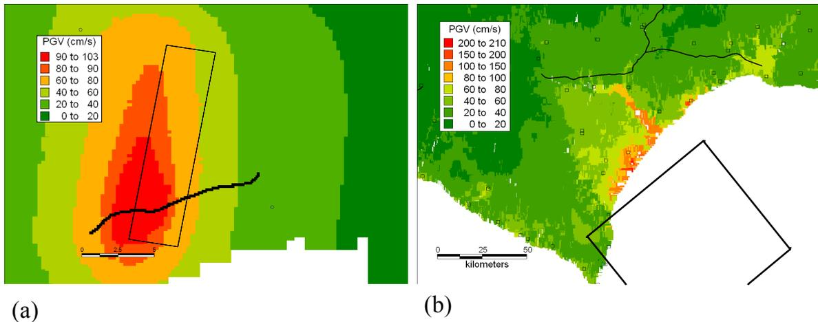
Figure 4 Estimated distribution of the peak ground velocity in (a) the 2003 Northern-Miyagi earthquake and (b) the 2003 Tokachi-oki earthquake
