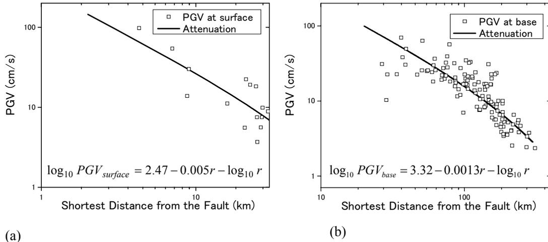
Figure 3 Attenuation relationship of PGV in (a) the 2003 Northern-Miyagi earthquake and (b) the 2003 Tokachi-oki earthquake
