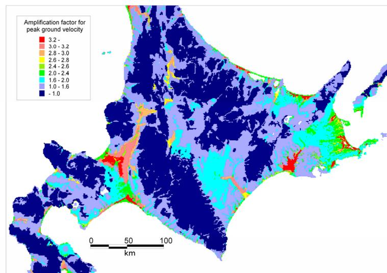
Figure 1 Amplification factors of the peak ground velocity in Hokkaido, Japan
