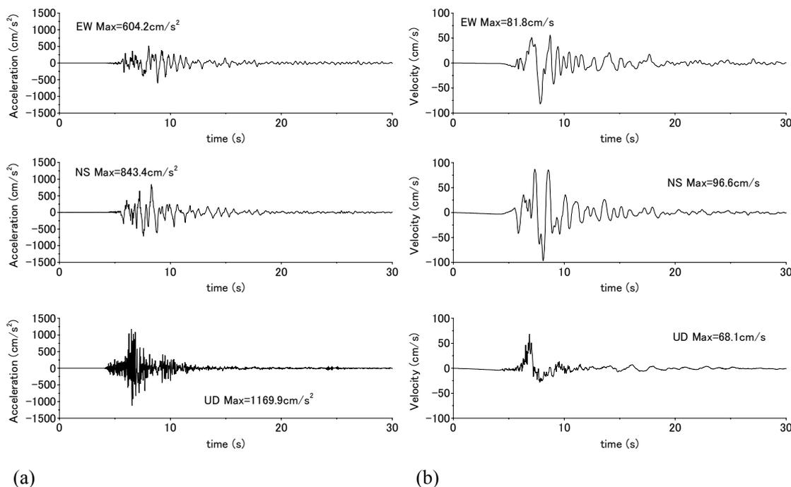
Figure 5 (a) Acceleration and (b) velocity time histories recorded at Yamoto IC during the 2003 Northern-Miyagi earthquake
