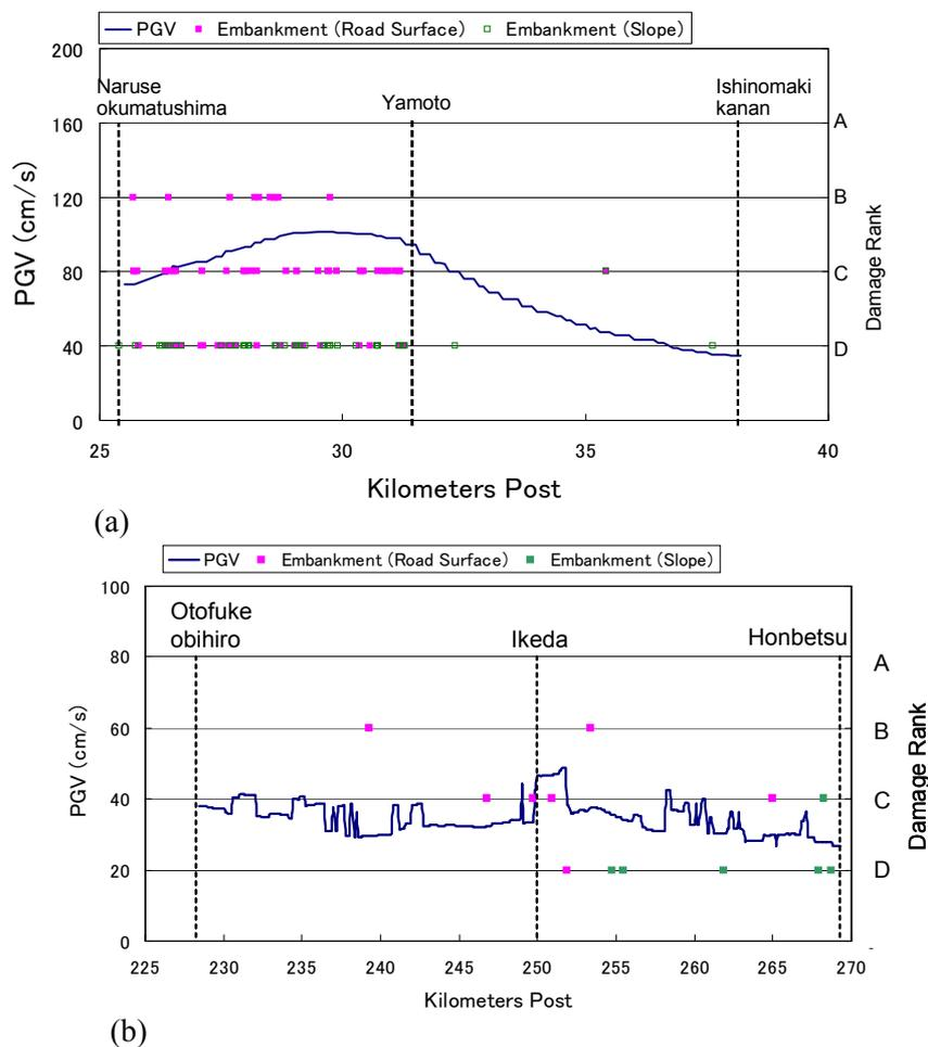
Figure 7 Relationship between the peak ground velocity and damages of expressway embankment for (a) the Sanriku expressway and (b) the Douto expressway embankment
