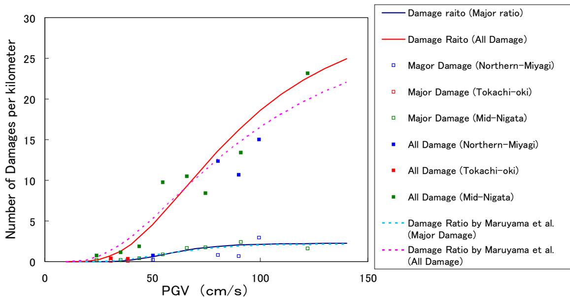
Figure 8 Fragility curves of expressway embankment with respect to the peak ground velocity
