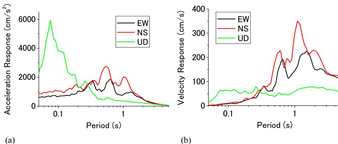
Figure 6 (a) Acceleration response spectra and (b) velocity response spectra with 5% damping ratio at Yamoto IC during the 2003 Northern-Miyagi earthquake
