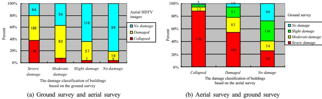
Figure 7: Relationship between the damage classifications for wooden buildings in Area 1 by two surveys
