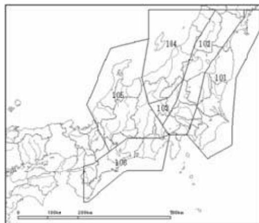
Fig. 6: Area source model for the North America Plate and Eurasia Plate
