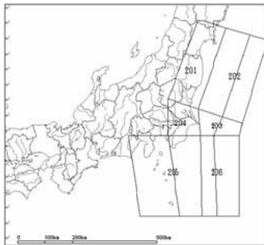
Fig. 5: Area source model for the Pacific Plate
