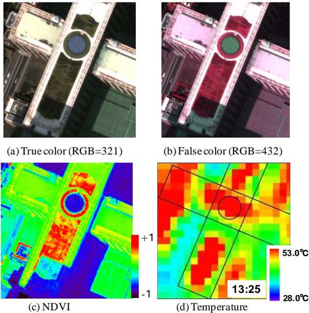
Figure 9. True color image (a), false color image (b), and NDVI image (c) by digital aerial camera, and the thermal image (d) of the rooftop of I-Hotel taken at 13:25, August 7, 2007 by TABI 320.
