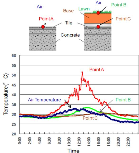
Figure 8. Measured temperatures on the rooftop of MLIT building on August 9, 2008 with the air temperature in central Tokyo [5].
