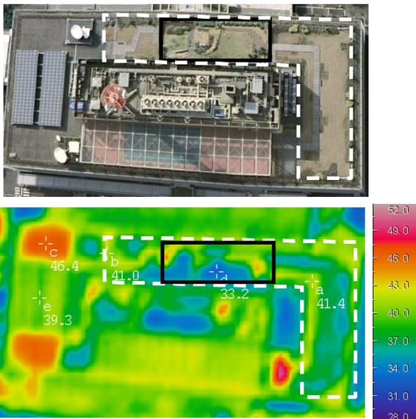
Figure 7. True color aerial image (top) and its thermal image (bottom) of the rooftop of MLIT building taken at 13:00, August 7, 2007 by Thermo Tracer TS7302.
