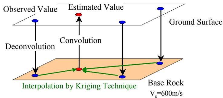
Figure 2. Schematic figure for interpolation of the peak ground velocity
