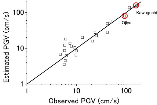
Figure 3. Comparison between the estimated peak ground velocity and the observed ones
