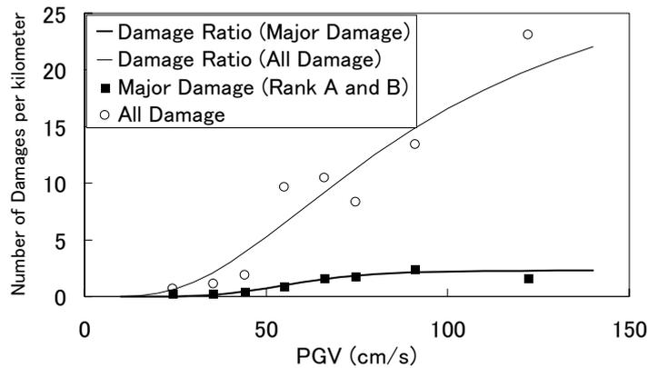
Figure 7. Fragility curves for expressway embankment with respect to the peak ground velocity
