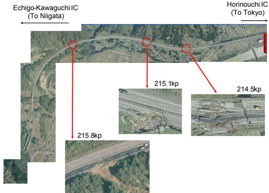
Figure 5. Post-earthquake aerial photograph of the Kanetsu Expressway showing severe damage at kilometre posts 215.8, 215.1, and 214.5
