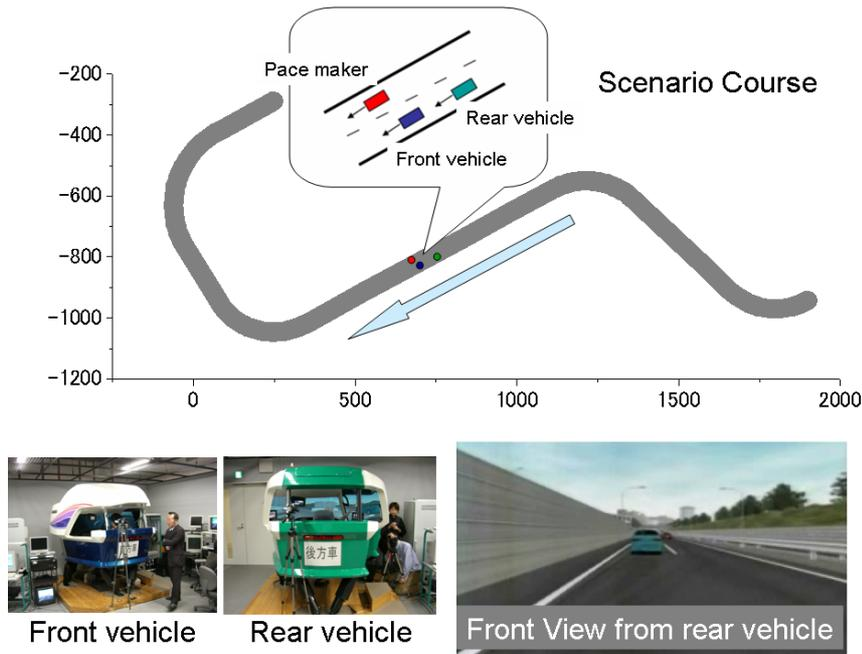
**Figure 1 Driving simulators used in this study and scenario highway course**
