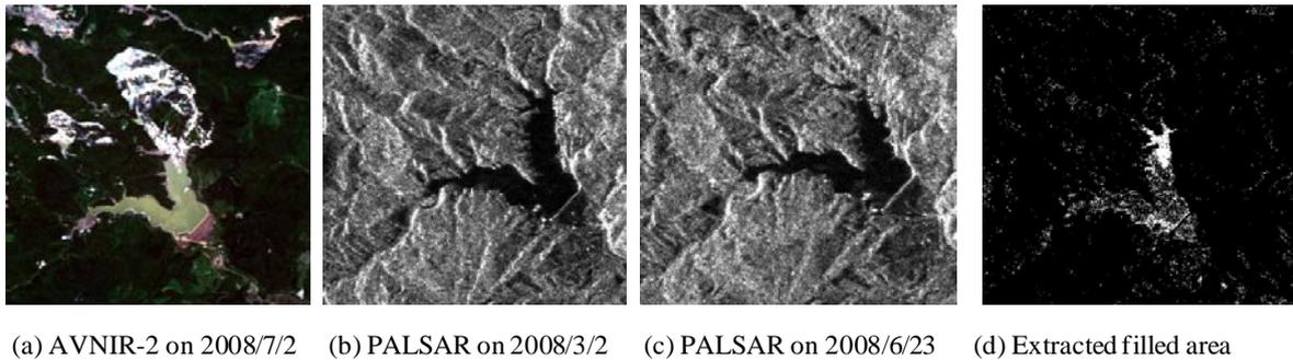
Fig. 2 ALOS/AVNIR-2 and PALSAR images including Aratozawa Dam. The filled area of water body (d) was extracted comparing the pre-event (b) and post-event (c) SAR images.
