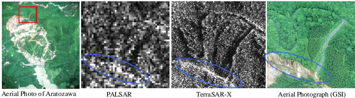
Fig. 3 Comparison of PALSAR and TerraSAR-X images with the aerial photograph (GSI, 2008)
