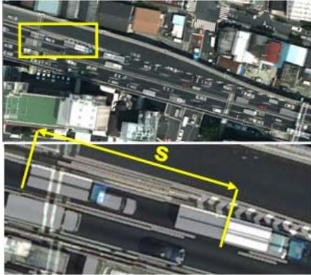
Fig. 6 Method of visual speed detection
