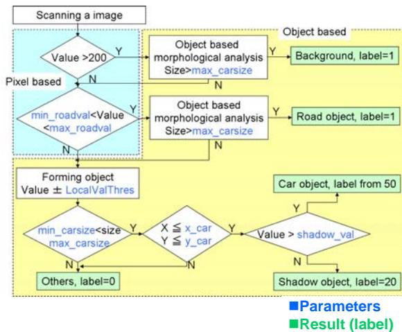
Fig. 3 Flowchart of the automated vehicle extraction
