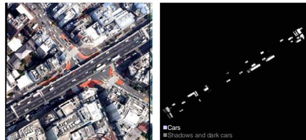
Fig. 5 Original image (left) and the result of vehicle extraction (right)
