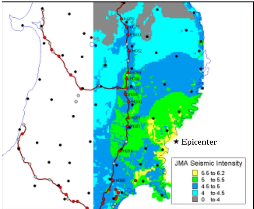
Figure 3. Estimated distribution of JMA seismic intensity on ground surface
