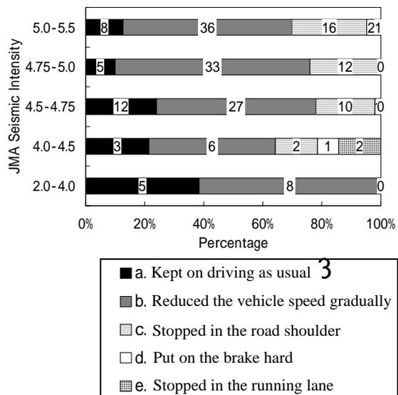
**Figure 8. Relationship between the JMA seismic intensity and the responses of drivers after the recognition of earthquake**
