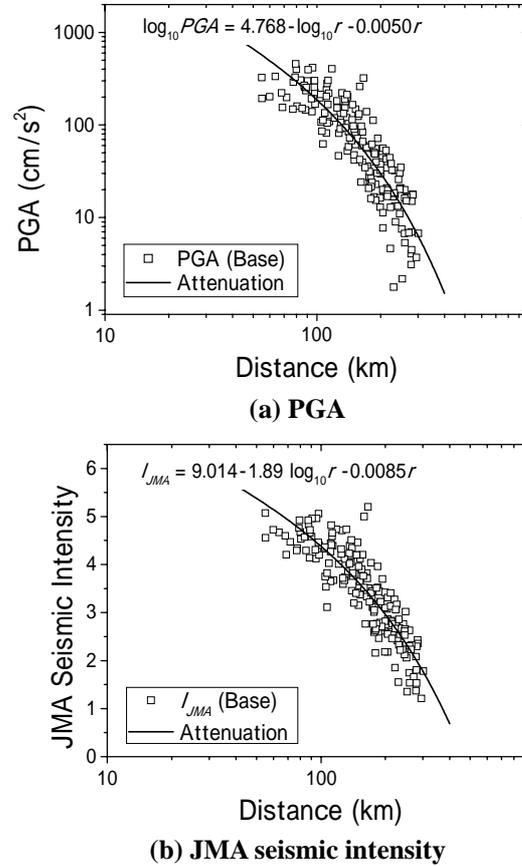
**Figure 2. Attenuation relationships of PGA and JMA seismic intensity at the base in the 2003 Sanriku-Minami earthquake**
