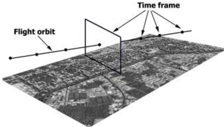
**Figure 4.** Illustration of determined flight orbit and time frames
