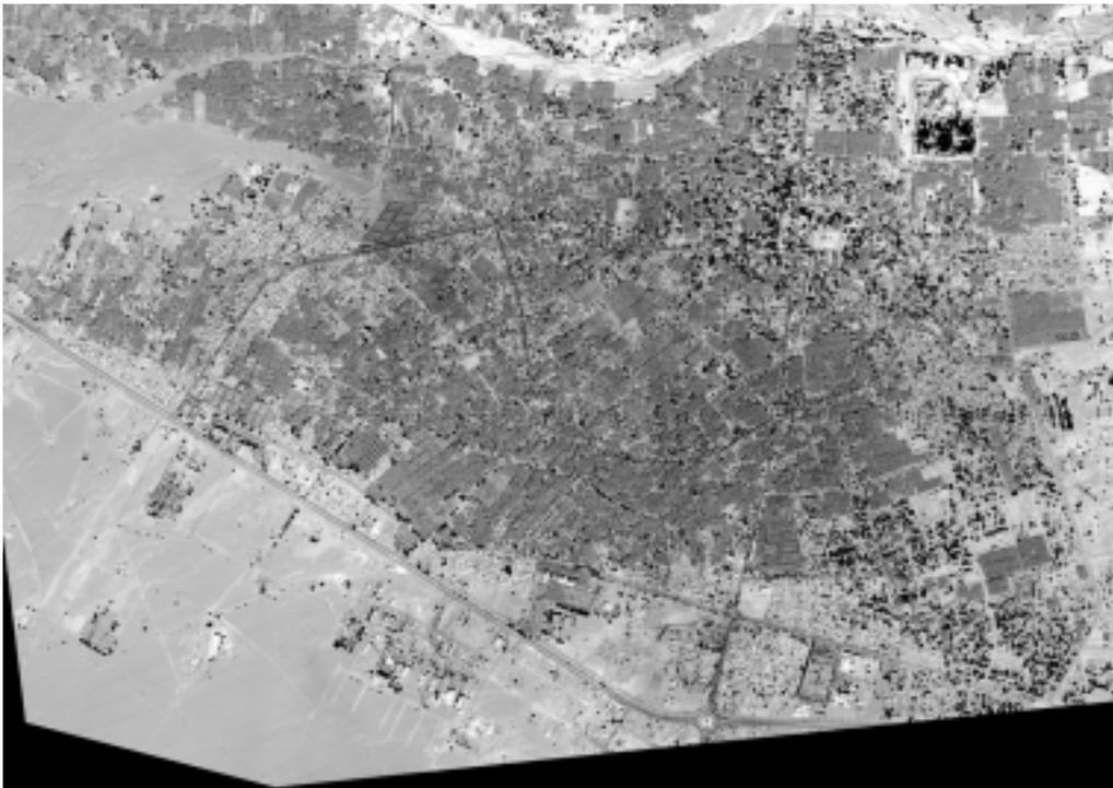
**Figure 3.** Distribution of detected damage areas in Bam city using color-modified QuickBird image.
