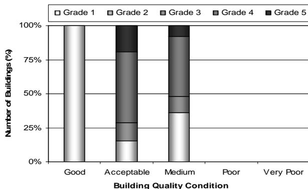
Figure 10. Damage Rank to Quality Class of selected buildings for M08.
