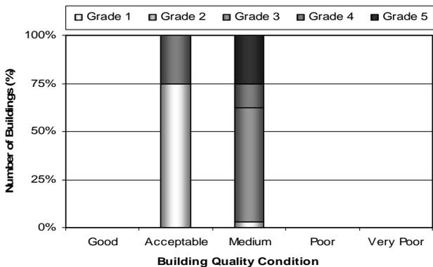
Figure 9. Damage Rank to Quality Class of selected buildings for M07.
