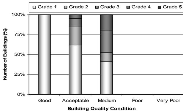
Figure 8. Damage Rank to Quality Class of selected buildings for M03.
