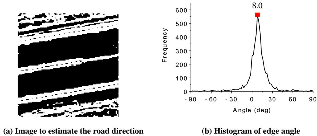
**Figure 6: Removal of road surface from the image and estimation of road direction**
