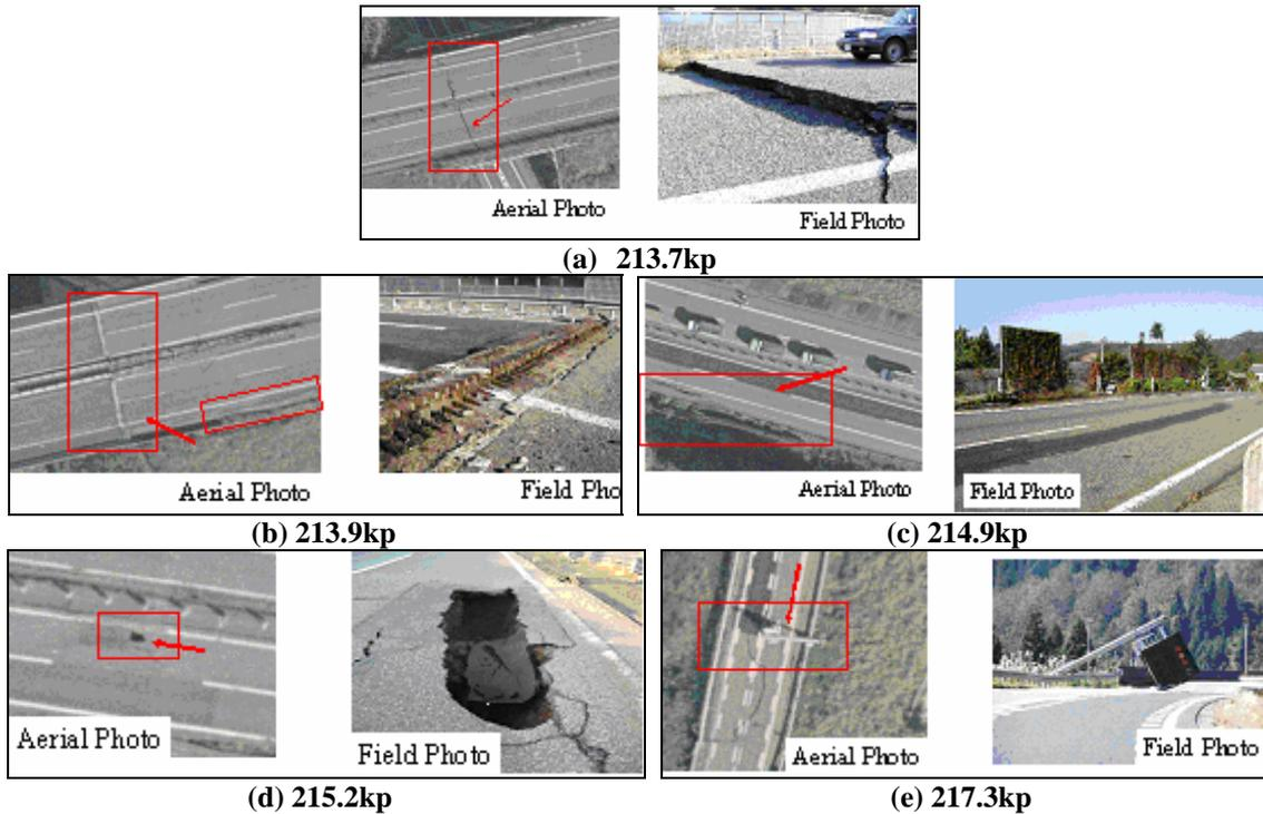
**Figure 2: Comparison of damages detected from the aerial photograph with those from field photographs**
