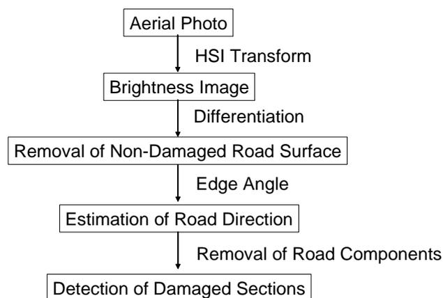
**Figure 4 : Flowchart of image processing to detect the damaged sections of expressways**
