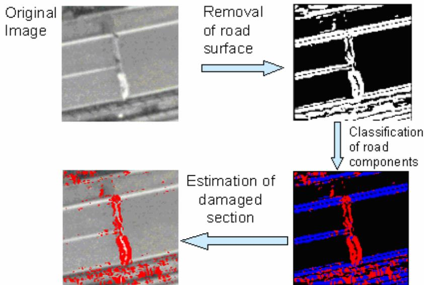
**Figure 7: Example of analytical flow to detect damaged sections of expressways**
