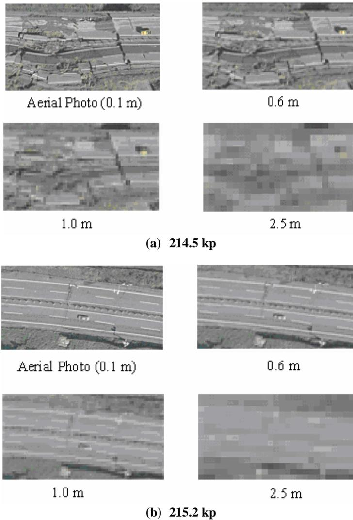
**Figure 3: Comparison of images which captured the damaged sections of the expressway with various resolutions**
