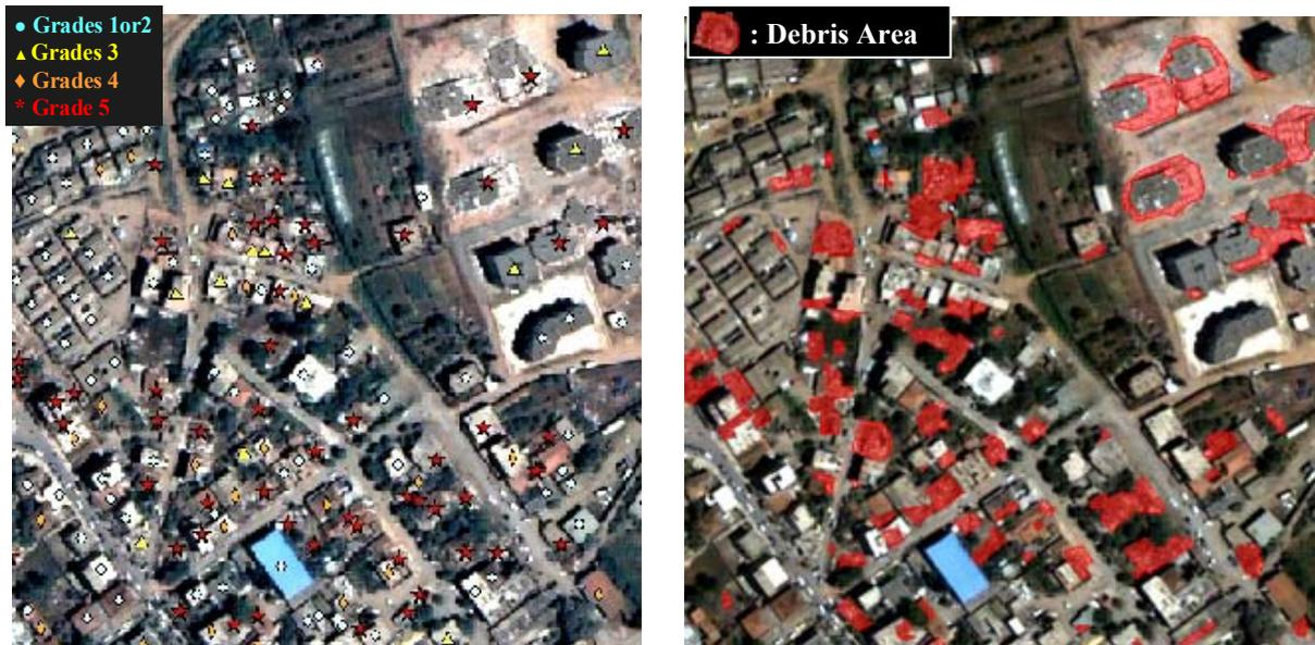
**Figure 4: (a) Result of visual building damage detection and (b) distribution of debris visually detected**
