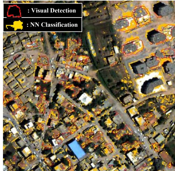
**Figure 5: (a) Debris detected by pixel-based approach and (b) debris detected by object-based approach**
