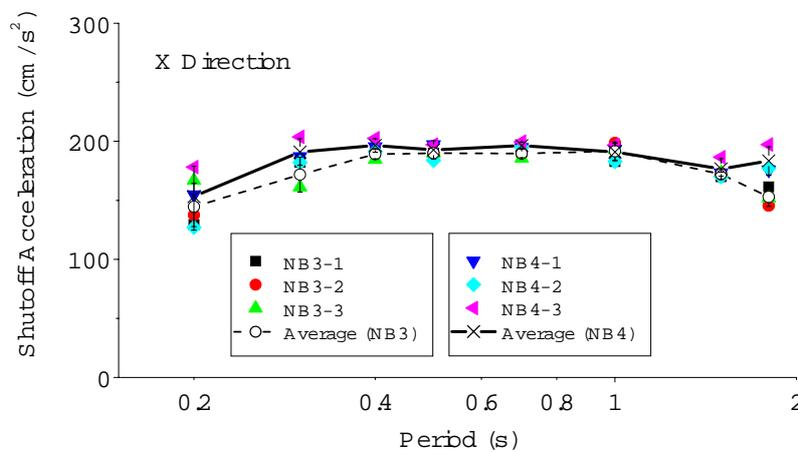
**Figure 4. Shutoff accelerations with respect to the periods of sinusoidal waves applied to the X direction**
