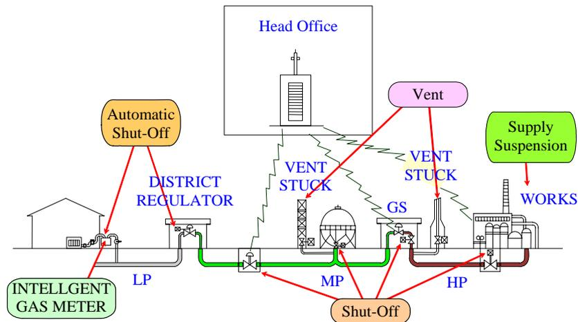
**Figure 1. Outline of emergency control of natural gas supply system in Japan**
