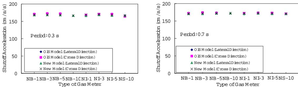
**Figure 2. Shutoff acceleration of various types of intelligent gas meters conducted by producteers (Old model: until February 2003, New model: from February 2003)**
