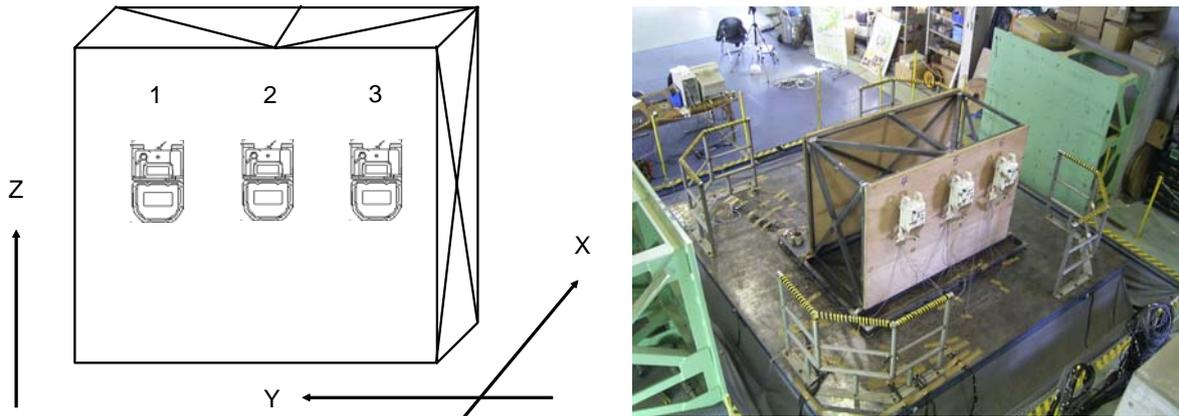
**Figure 3. Shaking table test of intelligent gas meters**
