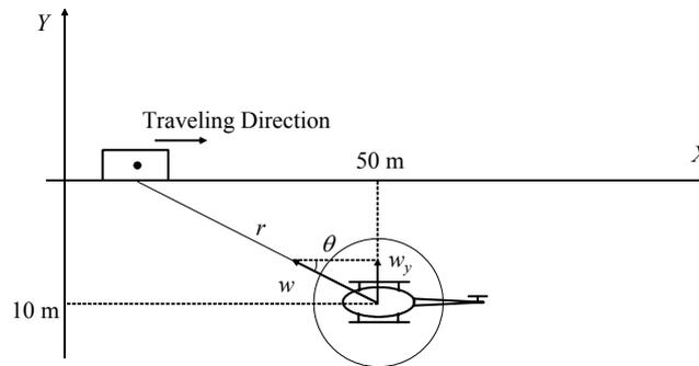
**Figure 5. Locations of a vehicle and a helicopter assumed in the numerical simulation**
