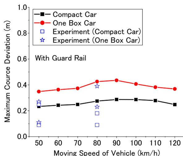
**Figure 7. Relationship between the moving speed of vehicles and maximum lateral displacements obtained from numerical simulations**
