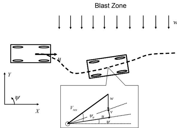
**Figure 4. Vehicle model and crosswind disturbance**
