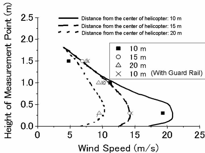
**Figure 3. Comparison between the wind velocity obtained from in this study and that from numerical simulation**
