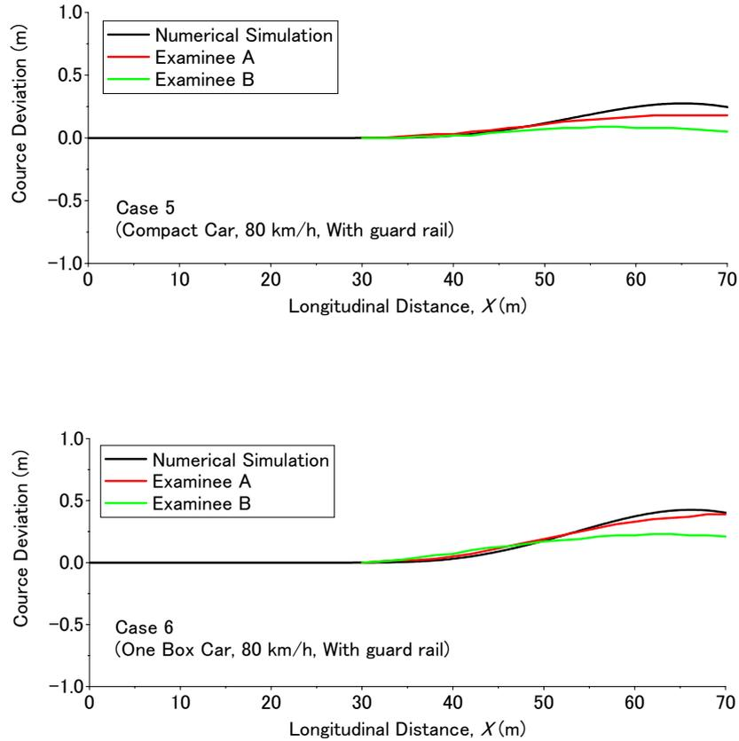
**Figure 6. Moving trajectories of vehicles obtained from actual driving tests and numerical simulation**
