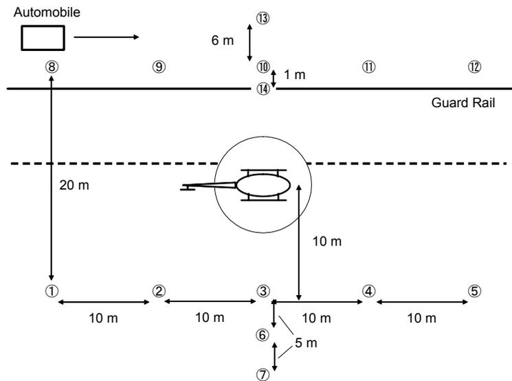
**Figure 1. Locations of anemometers in the wind velocity observation**
