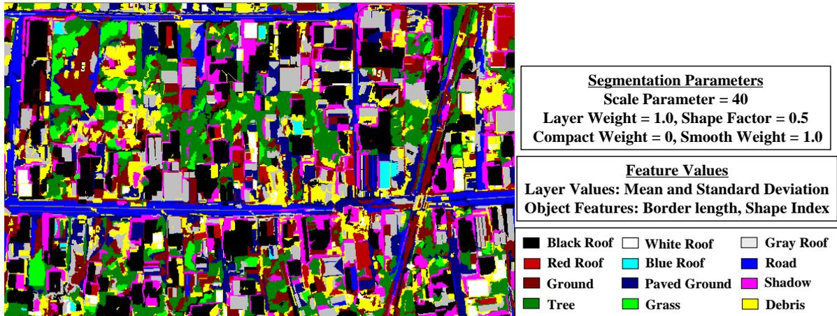
Figure 5 The result of object-based supervised classification and parameters used
