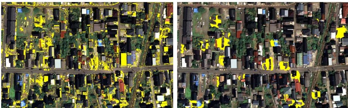
Figure 4 The results of automated damage extraction based on pixel-based classification (left) and visual inspection (right)
