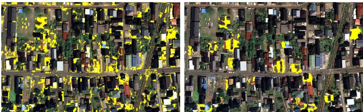
Figure 6 The results of automated damage extraction based on object-based classification (left) and visual inspection (right)
