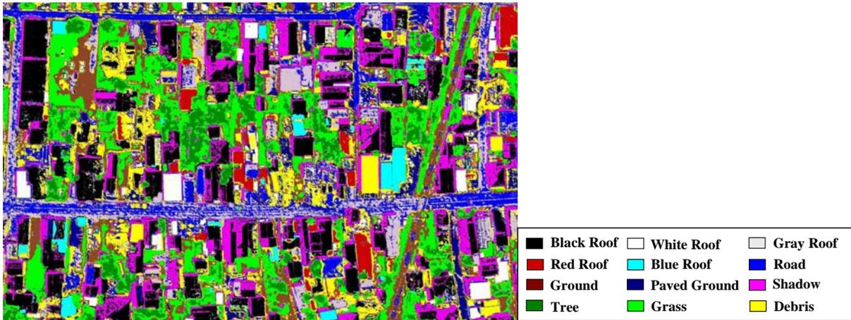
Figure 3 The result of pixel-based supervised classification
