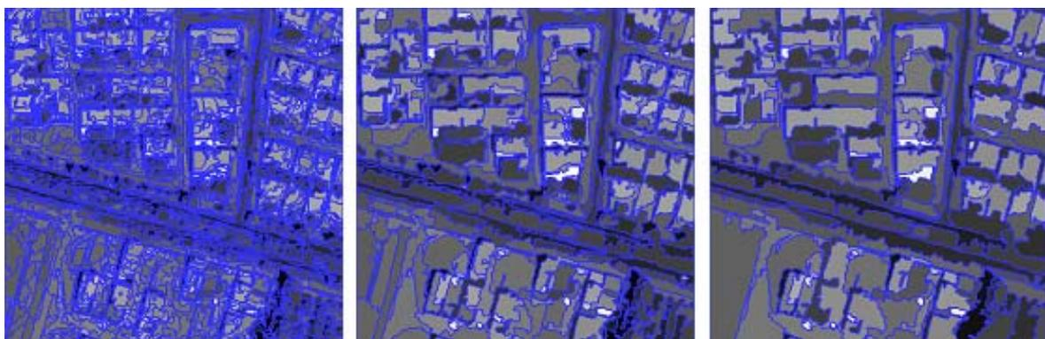
Figure 3. Difference of image segmentation by changing the scale parameter value (left:  $SP=10$ , center:  $SP=30$ , right:  $SP=50$ )
