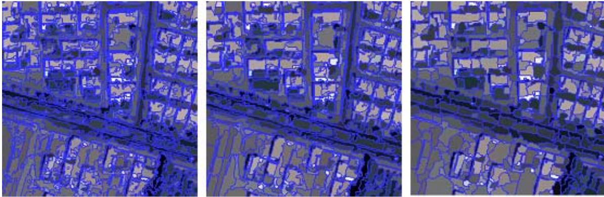
Figure 4. Difference of image segmentation by changing the shape factor value (left:  $SF=0$ , center:  $SF=0.2$ , right:  $SF=0.5$ )
