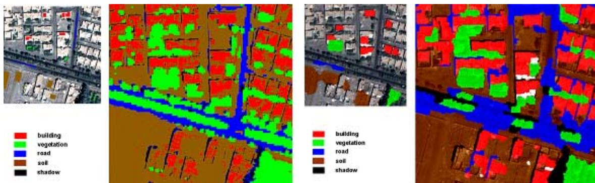
Figure 2. The original image with training data and the result of pixel-based classification (left) and object-based classification (right,  $w_{layer}=1.0$ ,  $SP=30$ ,  $SF=0.7$ )
