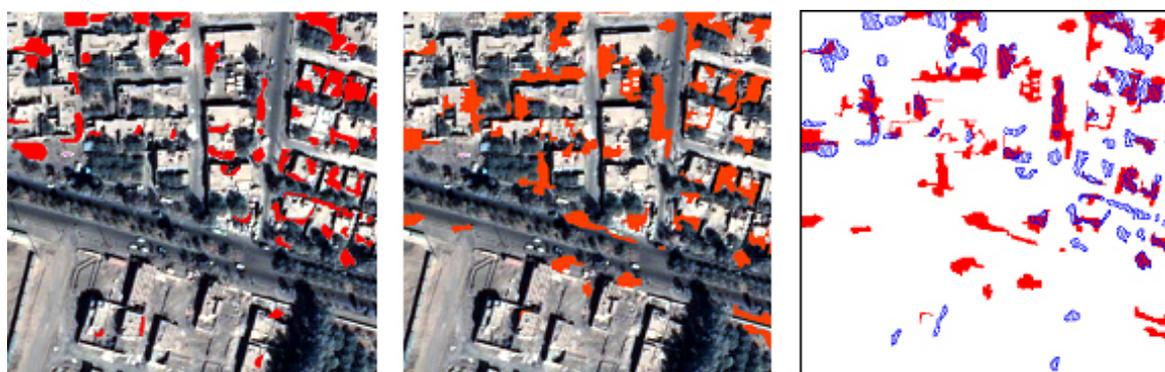
Figure 7. The visually detected (correct) area of debris (left), the classified area of debris (center), and the comparison of the two areas (right). (Red color is the true debris area and blue color is the classified area.)
