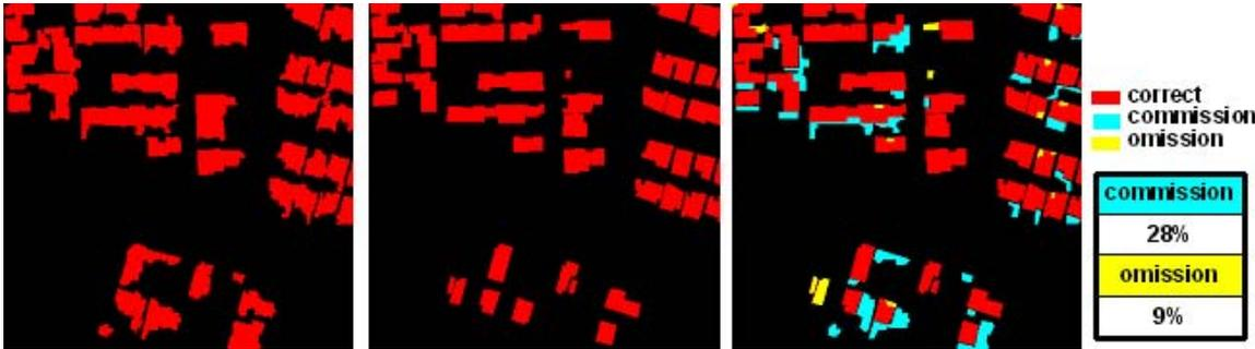
Figure 5. Results of object-based classification of buildings (left) and visual inspection (center) and comparison between these images (right).
