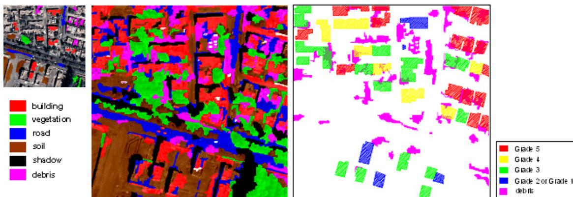
Figure 6. The original image with training data and the result of object-based classification (left,  $w_{layer}=1.0$ ,  $SP=20$ ,  $SF=0.5$ ) and the result of visual debris and building damage detection (right).
