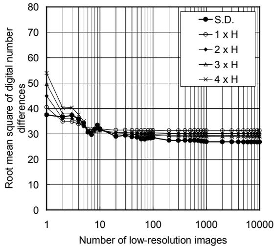
Figure 14 Number of low-resolution images and root mean square of digital number differences between synthesized image and reference image (parametric study on coefficients of filter  $H$ )
