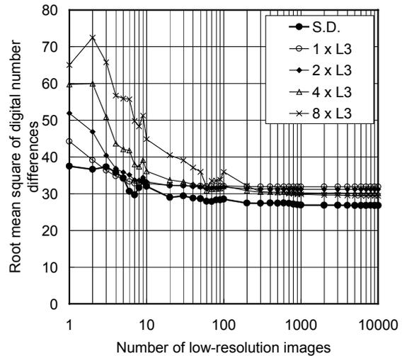
Figure 15 Number of low-resolution images and root mean square of digital number differences between synthesized image and reference image (3) (parametric study on coefficients of filter  $L_3$ )
