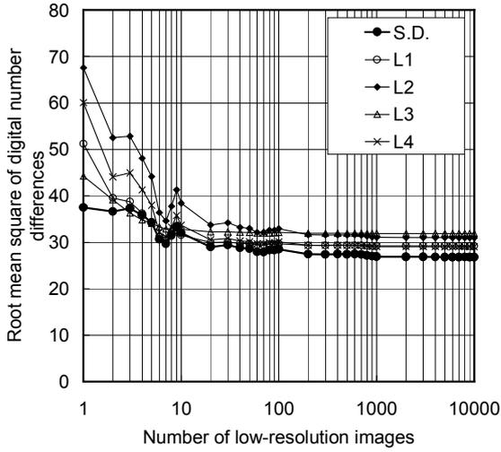
Figure 8 Number of low-resolution images and root mean square of digital number differences between synthesized image and reference image
