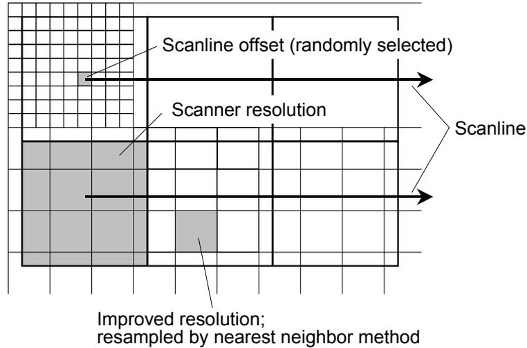
Figure 1 Randomly selected scanline offset and pixel division for resolution improvement
