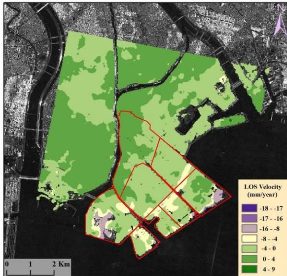
Figure 6. Estimated mean velocity of the LOS displacements from 2014 to 2017 using the SBAS-InSAR method from the ALOS-2 PALSAR-2 data.
