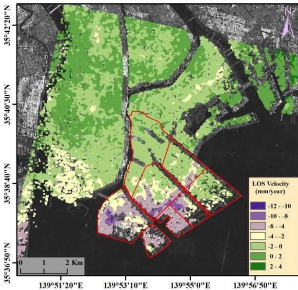
Figure 3. Estimated mean velocity of the LOS displacements from 1993 to 2006 using the SBAS-InSAR method from the ERS-1/-2 data.
