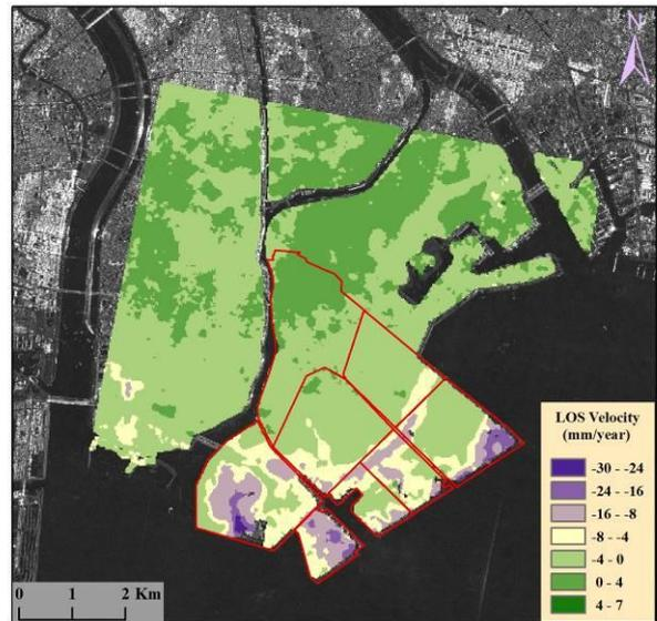
Figure 5. Estimated mean velocity of the LOS displacements from 2006 to 2011 using the SBAS-InSAR method from the ALOS PALSAR data.
