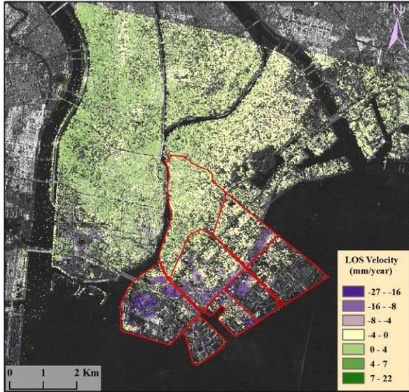
Figure 2. Estimated mean velocity of the LOS displacements from 1993 to 2006 using the PS-InSAR method from the ERS-1/-2 data.
