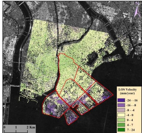
Figure 4. Estimated mean velocity of the LOS displacements from 2006 to 2011 using the PS-InSAR method from the ALOS PALSAR data.
