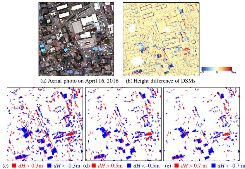
**Figure 7.** Aerial photograph around Mashiki Town office (a), height difference of the two DSMs (b), and extracted areas by different height-difference values (c-e). Objects smaller than  $9.0 \text{ m}^2$  were excluded.
