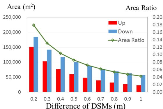
**Figure 5.** Relationship between the height difference and the area exceeding the plus and minus thresholds.
