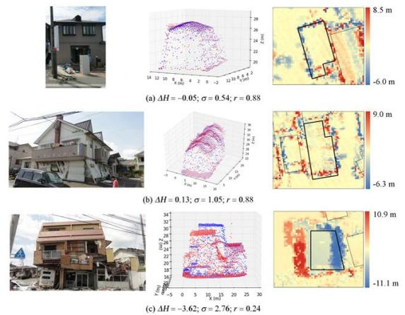
**Figure 3.** Examples of non-collapsed (a) and collapsed (b, c) buildings extracted using the Lidar data. The left figure shows the photos taken after the main-shock by the authors, the middle figure the two DSMs, and the right figure the elevation differences between the two DSMs..
