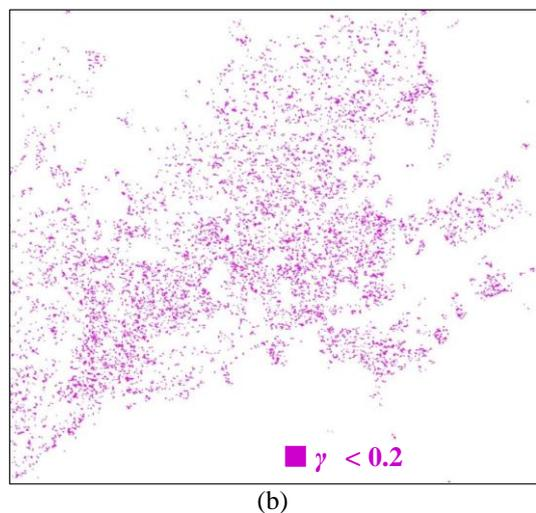
**Figure 6.** Changed areas extracted by height-difference (abs. (dH) > 0.5 m) of the two DSMs (a); and changed areas extracted by low coherence ( $\gamma < 0.2$ ) from PALSAR-2 data (b).
