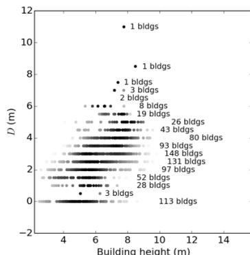
Figure 2. Scatter plot of debris extent ( $D$ ) and building height.
