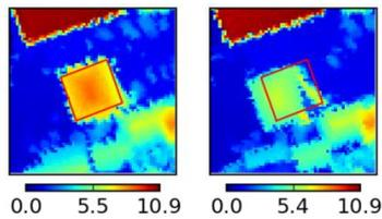
Figure 1. Closer look of a building. Left: pre-event DSM. Right: post-event DSM.
