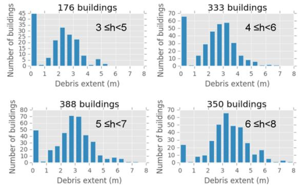
Figure 3. Histogram of debris extent of collapsed buildings grouped by ranges of height.
