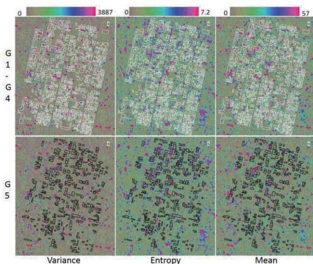
**Figure 6.** GLCM features to be used as indicators in building damage extraction for the entire study area: (a) variance, (b) entropy, (c) mean.
