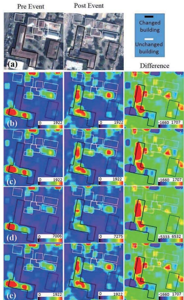
**Figure 3.** Change situation of GLCM variance in a sample area: (a) the pre- and post-event optical images, (b) the standard index, (c) displacement change, (d) grey-level change, (e) direction change.
