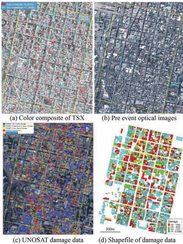
**Figure 2.** The target area: (a) color composite of TSX, (b) the pre-event QuickBird, (c) the post-event WorldView-2 image with the damage data by UNOSAT, (d) shapefile created by Miura et al. (2012).
