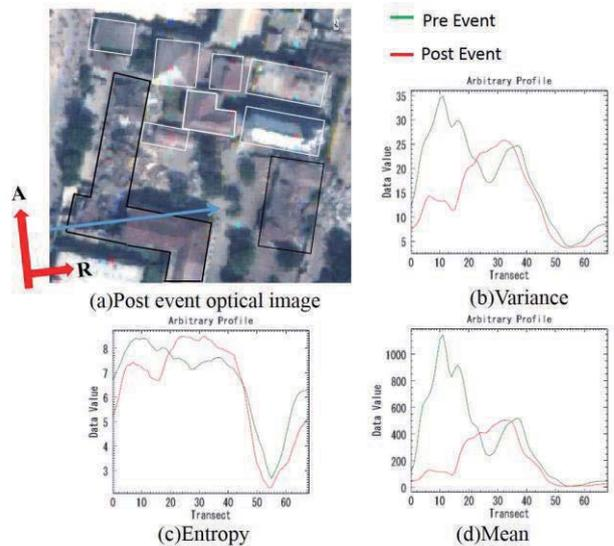
**Figure 5.** Examination of collapsed buildings by Profile Line: (a) Post event optical images with profile line, (b) Variance, (c) Entropy, (d) Mean.
