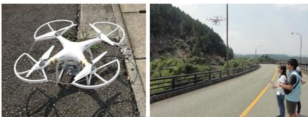
**Fig. 2** Phantom 3 Professional UAV used in this study (left) and a scene of manual flight (right)
