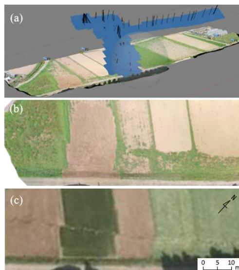
**Fig. 3** Surface faulting in Dozono district, Mashiki town: Developed 3D model with estimated camera positions (a), an orthomosaic image made by SfM (b), and the ortho-photo made by GSI, taken on April 29 (c).
