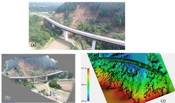
**Fig. 5** A still-photo from UAV (a), 3D model (b), and DSM (c) created by SfM for Ohkiri-hata bridge area.
