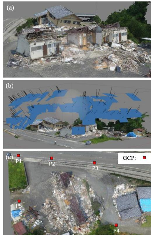
**Fig. 6** Developed 3D model of collapsed buildings in Kawayo district (a), 3D model with estimated camera positions (b), and the layout of GCPs (c)
