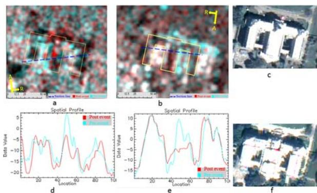
Figure 7. Non-individual building with three wings in the colour composites of the ascending (a) and descending (b) TSX intensity images with the section lines; the backscatter intensity values along the section lines in the ascending (d) and descending (e) pairs; the pre- (c) and post-event (f) optical images of the target building.
