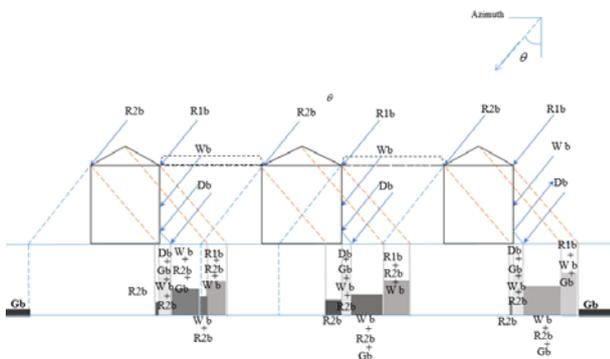
Figure 5. Schematic representation of non-individual building with the gable-roof in a SAR image including the details of layover
