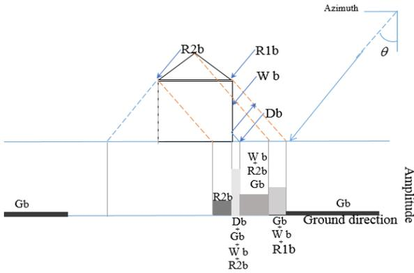
Figure 4. Schematic representation of an individual building with gable-roof in the SAR image including the details of layover.
