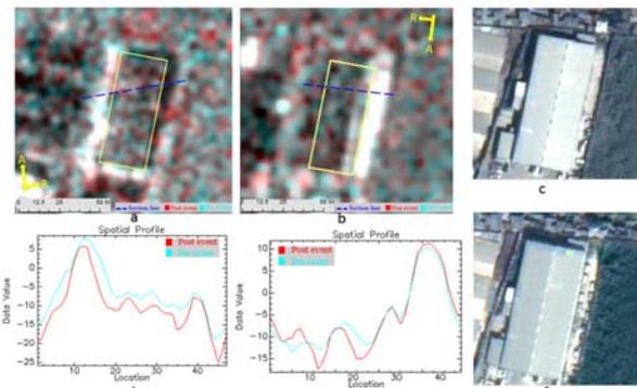
Figure 6. Individual building with the gable-roof in the colour composites of the ascending (a) and descending (b) TSX intensity images with the section lines; the backscatter intensity values along the section lines in the ascending (d) and descending (e) pairs; the pre- (c) and post-event (f) optical images of the target building.
