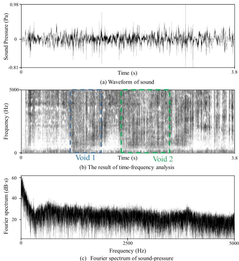
Figure 5. Recorded sound by rotary hammer along the line  $\alpha\text{-}\alpha'$  in the retaining wall.
