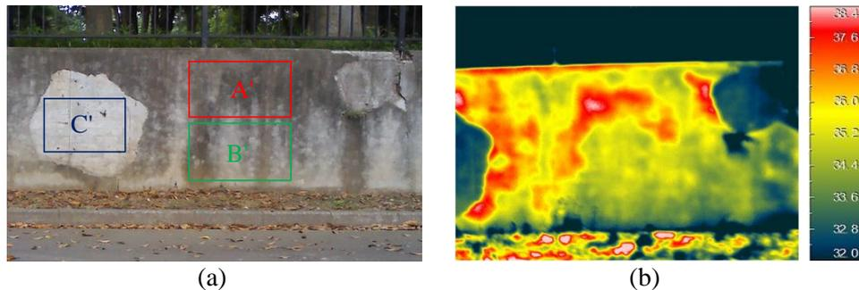
Figure 8. The measured data on June 27, 2013. (a) The measurement area by Schmidt hammer and (b) the thermal image.
