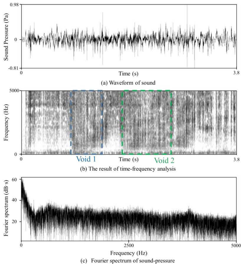
Figure 5. Recorded sound by rotary hammer along the line  $\alpha$ - $\alpha'$  in the retaining wall.
