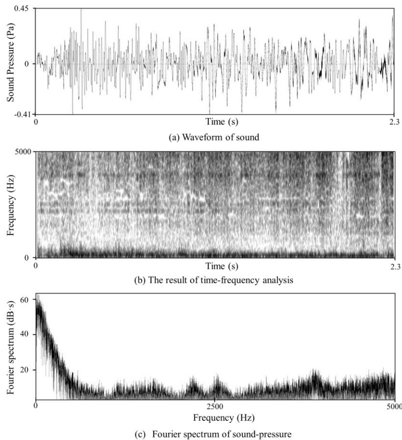
Figure 6. Recorded sound by rotary hammer along the line  $\beta$ - $\beta'$  in the retaining wall.
