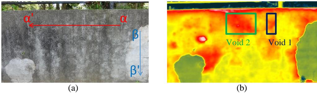
Figure 4. (a) The measurement area of rotary hammering test (line  $\alpha$ - $\alpha'$  and  $\beta$ - $\beta'$ ) and (b) the thermal image at 15:30.
