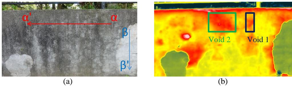
Figure 4. (a) The measurement area of rotary hammering test (line  $\alpha\text{-}\alpha'$  and  $\beta\text{-}\beta'$ ) and (b) the thermal image at 15:30.
