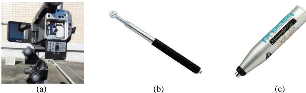
Figure 1. Instruments used in this study. (a) Infrared thermography camera (Nippon Avionics Co., Ltd. (2014), InfReC R300SR-SS), (b) Rotary hammer (Dogyu Sangyo Co. (2014), No. 01738), and (c) Schmidt hammer (Fuji Bussan Co. (2014), Type N).
