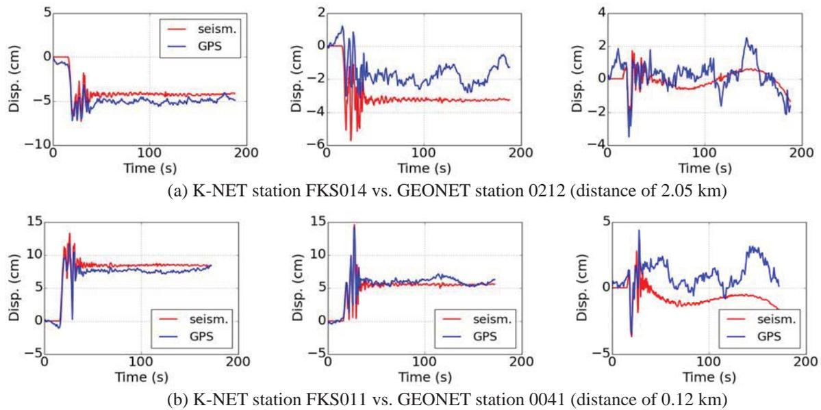
Figure 7. Comparison of coseismic displacements from GPS and acceleration records in the 2011 Fukushima event at the stations in Figure 6 to the EW (left), NS (middle), and UD (right) directions
