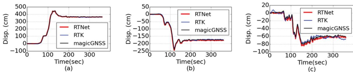
Figure 2. Displacement solutions of the Tohoku earthquake using PPP technique for GEONET Kesennuma (0172) station during the 2011 Tohoku event; EW (a), NS (b) and UD (c) components
