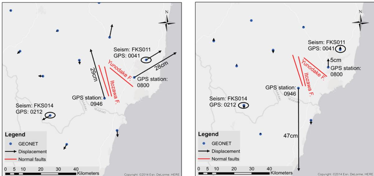
Figure 6. Coseismic displacement distribution due to the 11 April 2011 Fukushima earthquake to the horizontal (left) and vertical (right) directions calculated from GEONET data.
