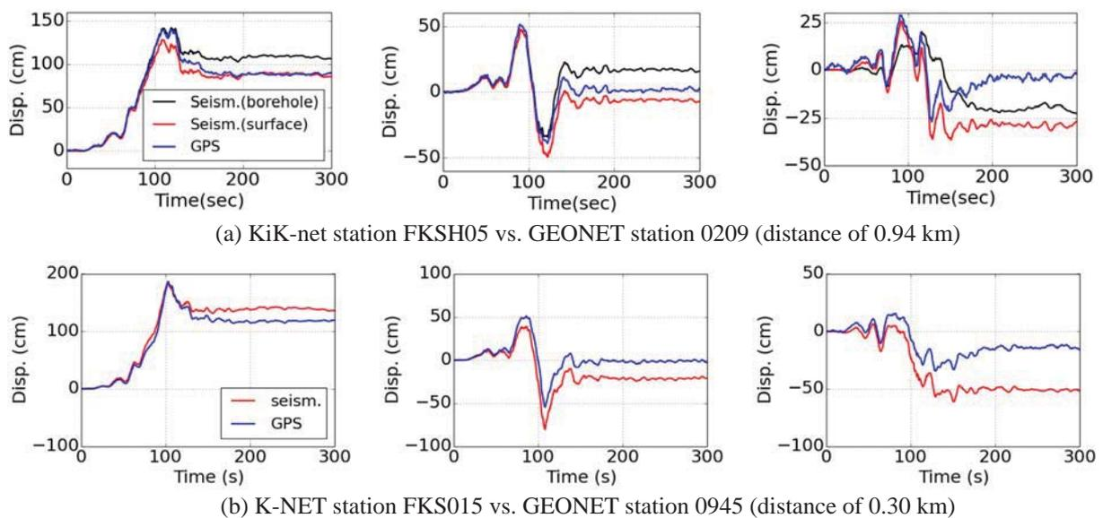
Figure 5. Comparison of coseismic displacements from GPS and acceleration records during the 2011 Tohoku earthquake at the stations in Figure 4 to the EW (left), NS (middle), and UD (right) directions
