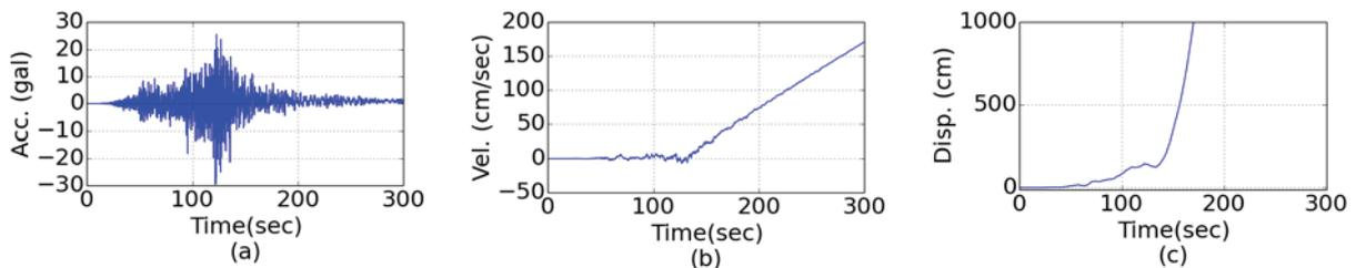
Figure 1. Direct double integration without baseline correction for a KiK-net FKSH04 station record (2011/3/11) in the EW direction; acceleration (a), velocity (b) and displacement (c)
