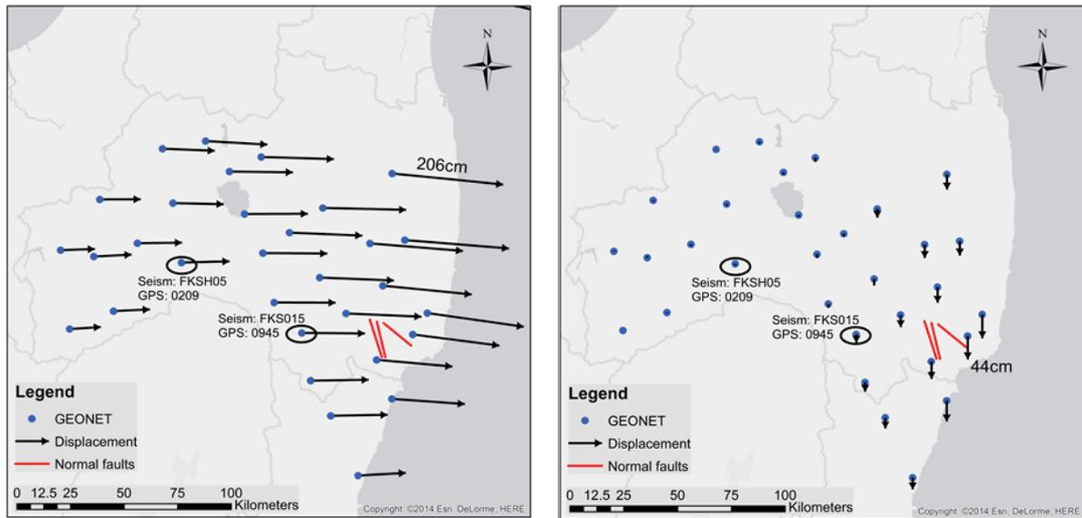
Figure 4. Coseismic displacement distribution due to the 11 March 2011 Tohoku earthquake to the horizontal (left) and vertical (right) directions calculated from GEONET data
