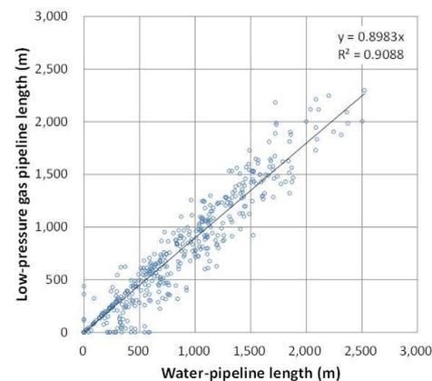
Figure.9. Relationship between water and gas pipeline lengths in 250m grid cells in Kashiwazaki.
