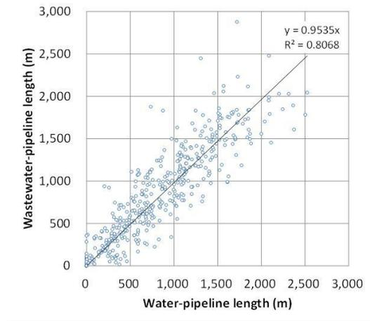
Figure.8. Relationship between water pipeline and wastewater line length in 250m grid in Kashiwazaki.
