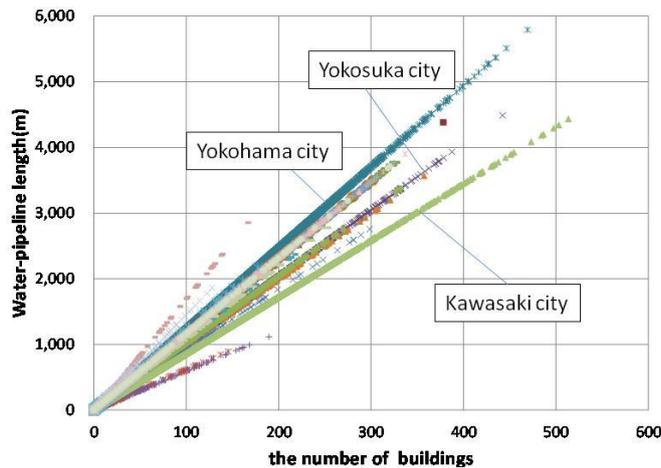
Figure.1. Comparison of the number of buildings and water pipeline lengths in 250m grid cells for cities in Kanagawa prefecture.
