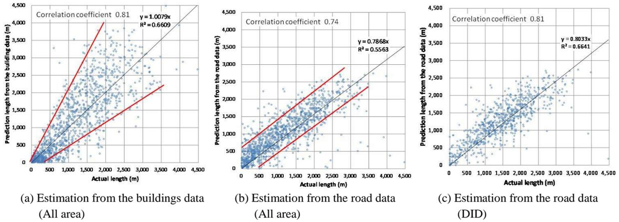
Figure.5. Comparison of actual and predicted water pipeline lengths in 250m grid cells (in Kanagawa).
