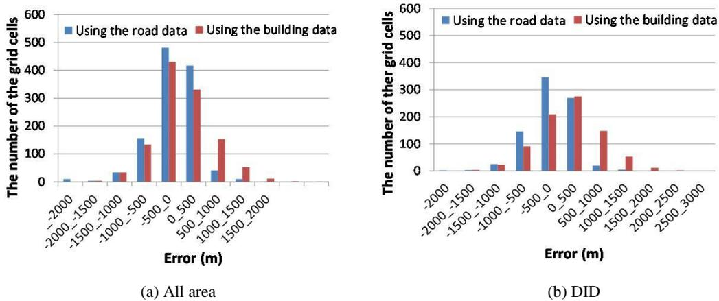
Figure.6. Comparison of errors between the actual and predicted water pipeline lengths in the city in Kanagawa prefecture from the road data and the building data.
