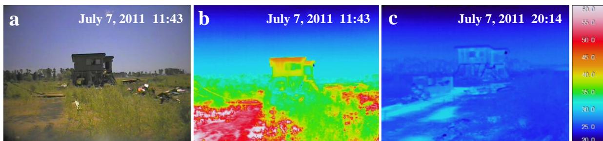
Figure 6. a: Optical image of daytime, b,c: Thermal infrared images of daytime and nighttime (Unit: °C). A house in a tsunami affected area is shown.
