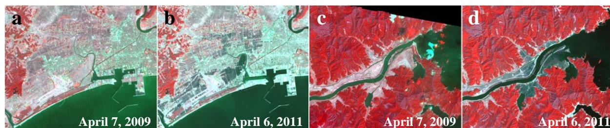
Figure 4. a,b: False color composite of the images before and after the earthquake in (1), c,d: that in (2).
