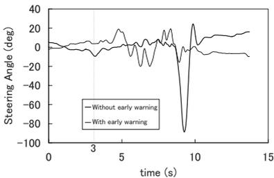
Figure 17. Comparison of the steering angles of the examinees with/without early warning of seismic motion.
