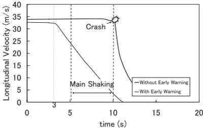
Figure 16. Comparison of the moving speeds of the examinees with/without early warning of seismic motion.
