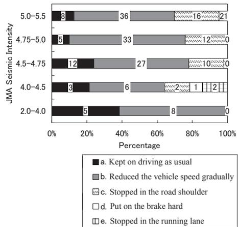
Figure 3. Relationship between the JMA seismic intensity and the responses of drivers after the recognition of earthquake.
