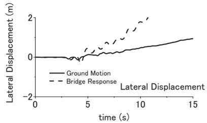
Figure 8. Comparisons between responses of the vehicle under the ground motion and those under the response of bridge pier. (Input ground motion is JMA Kobe record.)
