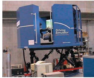
Figure 10. Driving simulator used in this study.
