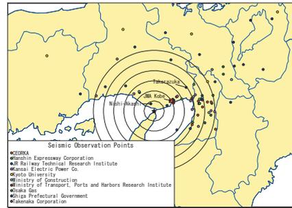
Figure 13. Locations of seismic observation points and epicenter in the 1995 Kobe earthquake. (The distance between each adjacent circle is 10 km.)
