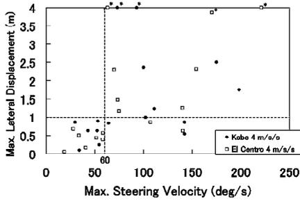
Figure 12. Relationship between the maximum lateral displacement of the moving vehicle and the maximum steering velocity. (The points with \* are the results from the examinees who moved to the adjacent lane during an earthquake.)
