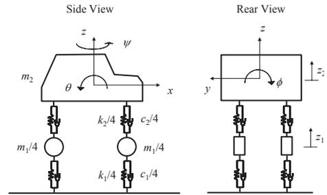
Figure 4. Vehicle model with a six-degree-of-freedom system used in this study.
