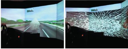
Figure 14. Example of the driving simulator experiment to avoid the obstacle during an earthquake without early warning of seismic motion. (crashed in the obstacle.)
