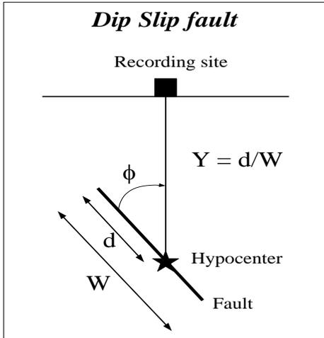
Figure 2. Definition of rupture directivity Parameters.
