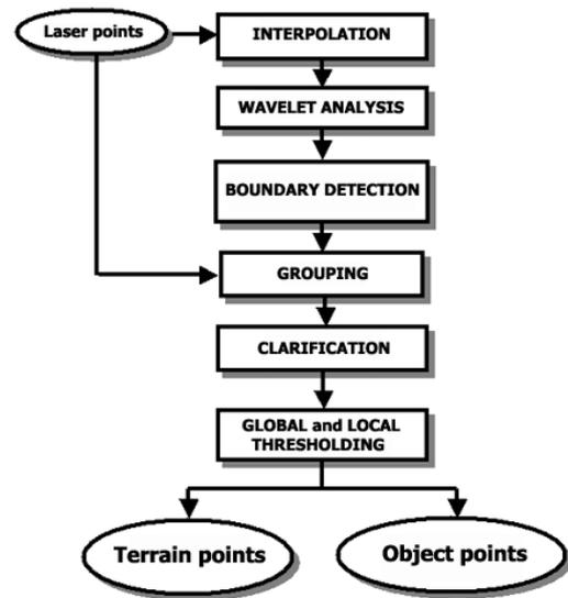
Figure 1. The components of the processing system
