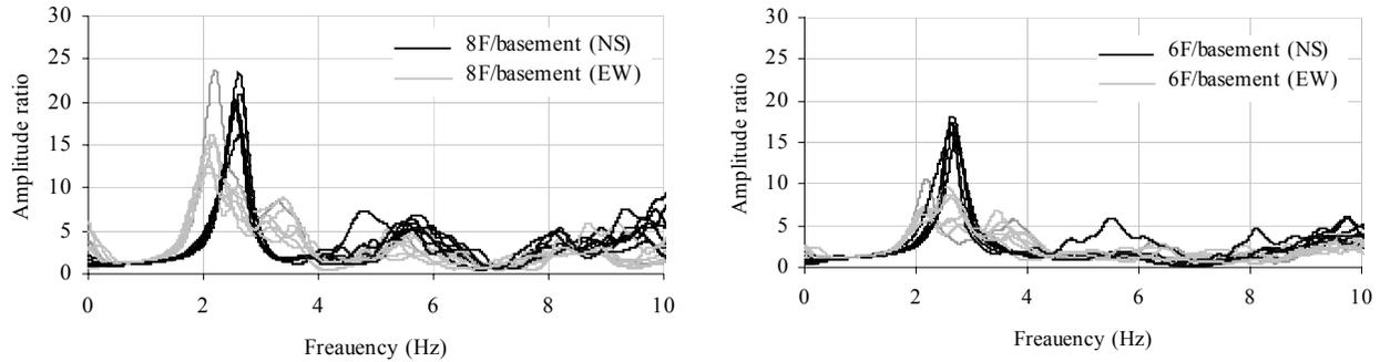
Figure 9. Fourier spectral ratios between the 8th floor (west wing) or 6th floor (east wing) and basement for the 6 seismic events.
