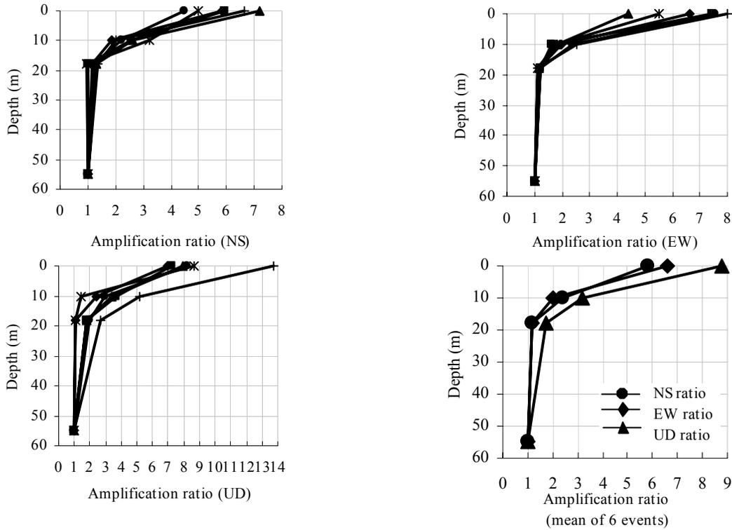
Figure 4. Amplification ratios of peak acceleration
