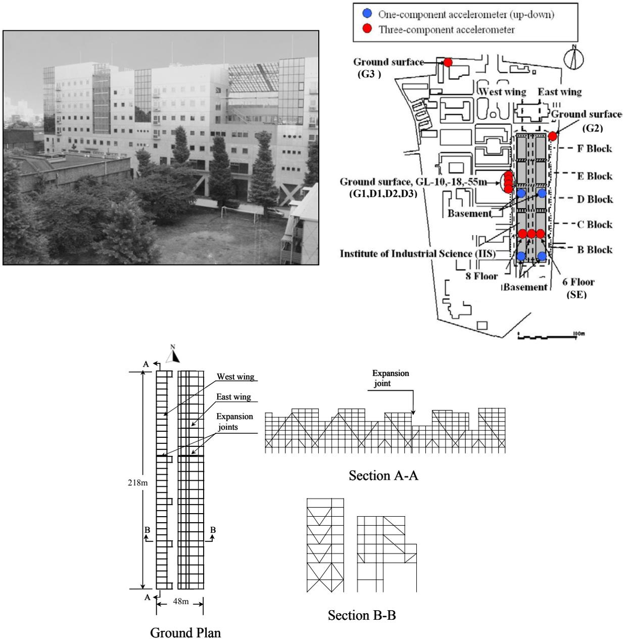
Figure 2. The Institute of Industrial Science Building and location of accelerometers
