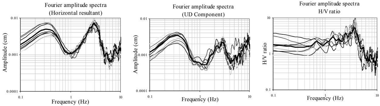
Figure 6. Fourier spectra of 10 time windows of microtremors and their average at the location of accelerometer G3.
