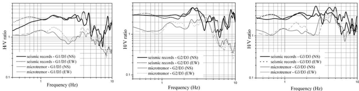
Figure 7. H/V Fourier spectral ratios of seismic ground motions and microtremors at G1, G2, and G3 accelerometer's location.
