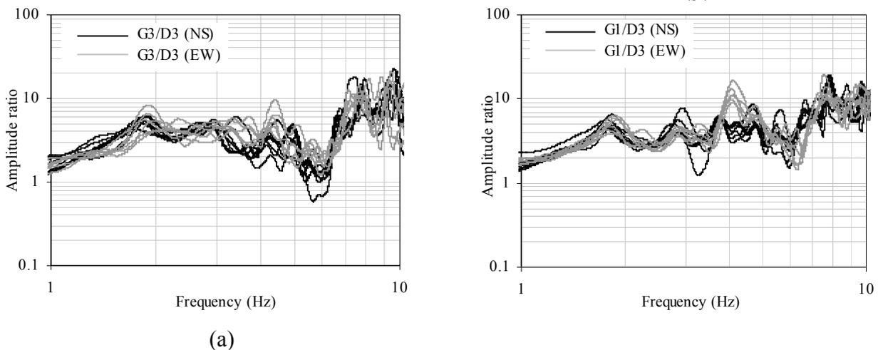
Figure 5. Transfer functions of the seismic records in the NS and EW components. (a) between G3 and D3 and (b) between G1 and D3.
