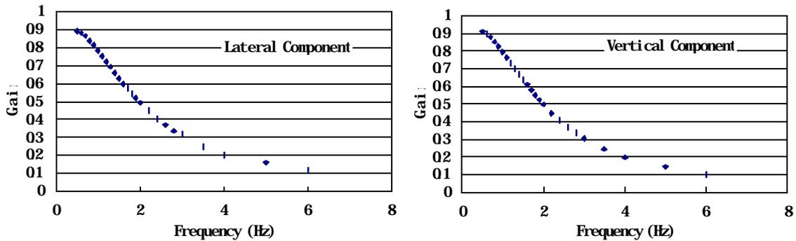
Figure 8. Amplitude ratio between the motion produced by the actuators and the motion applied to the actuators
