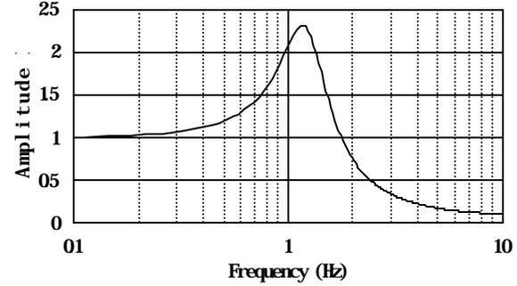
**Figure 3. Response characteristics of a vehicle to vertical motion**
