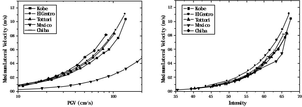
Figure 6. Relationship between the maximum lateral velocity of the vehicle and the peak ground velocity applied to the transverse direction to the vehicle (left) and the relationship between the maximum lateral velocity of the vehicle and JMA intensity (right)
