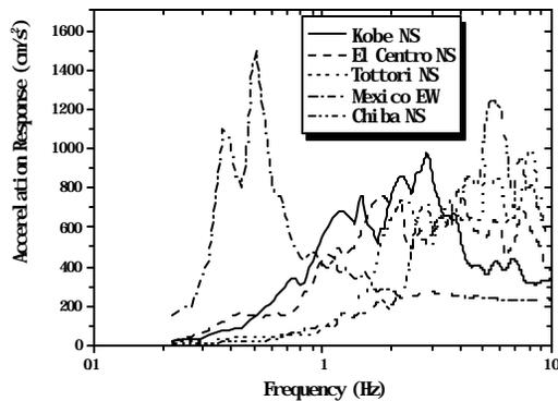
**Figure 4. Acceleration response spectra (5 % damping) of five records scaled to  $\text{PGA}=300\text{cm/s}^2$  applied to the transverse direction to the vehicle**
