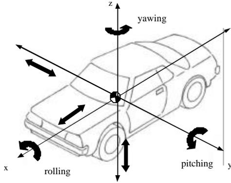
Figure 1. Fundamental motions of a vehicle
