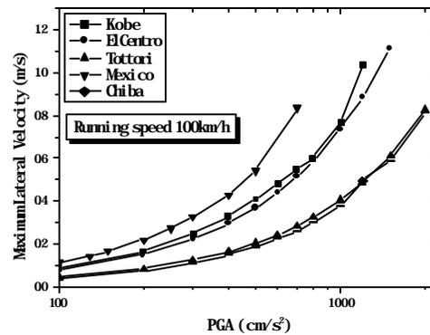
**Figure 5. Relationship between the maximum lateral velocity of the vehicle and the peak ground acceleration applied to the transverse direction to the vehicle**
