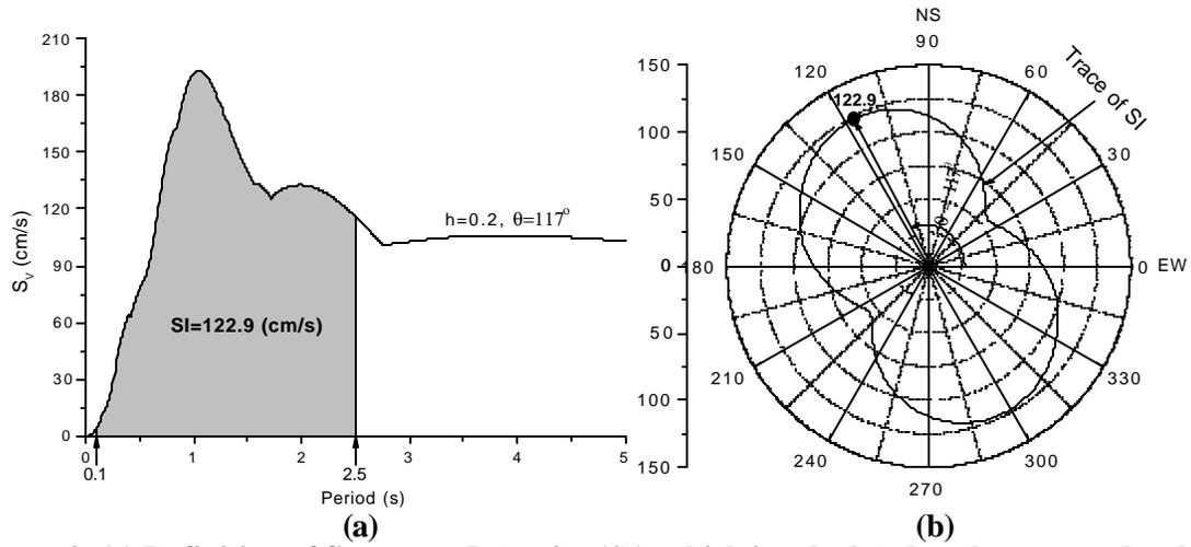
**Figure 2. (a) Definition of Spectrum Intensity (SI), which is calculated as the area under the relative-velocity response spectrum with 20% damping ratio between the periods of 0.1s and 2.5s, divided by the period interval, and (b) trace of SI, which is computed from the EW and NS components of acceleration records of the JMA Kobe station of the 1995 Kobe earthquake. The maximum value of SI is shown on the trace with a solid circle, which is obtained at  $q=117^\circ$ .**
