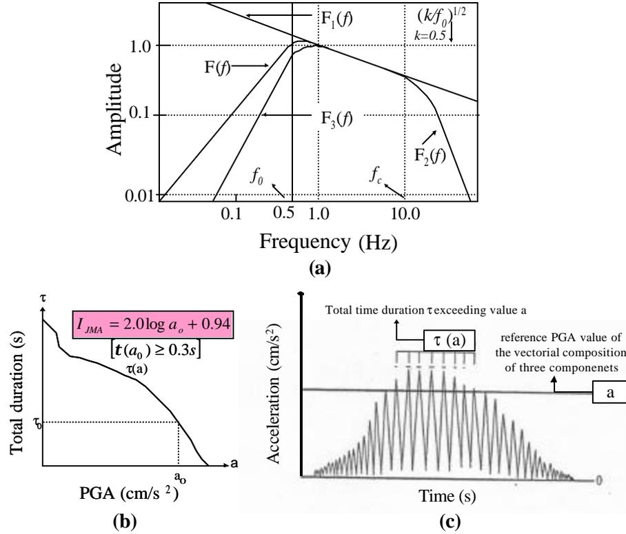
**Figure 1. Calculation of JMA instrumental seismic intensity, which is obtained by (a) applying a band pass filter in the frequency domain and (b) considering the durational effect  $t(a)$  of PGA, which is obtained in the time domain by (c) summing the time segments exceeding a reference PGA value of the vectorial composition of the three-components of acceleration records.**
