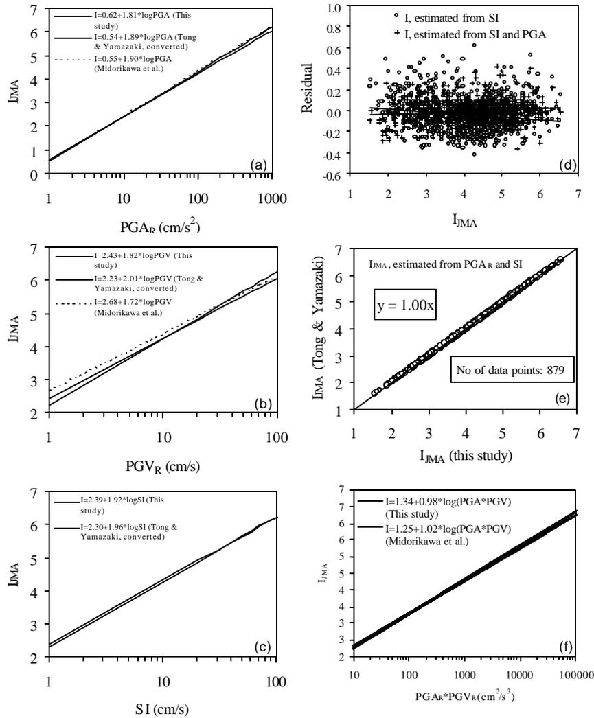
**Figure 3. Comparison of the relationships between the JMA seismic intensity and ground motion indices obtained in this study with the ones obtained by other studies [5, 6]. The plots of the residuals of  $I_{JMA}$  obtained from single and multiple ground motion indices are also shown in the figure (d) at the top right corner.**
