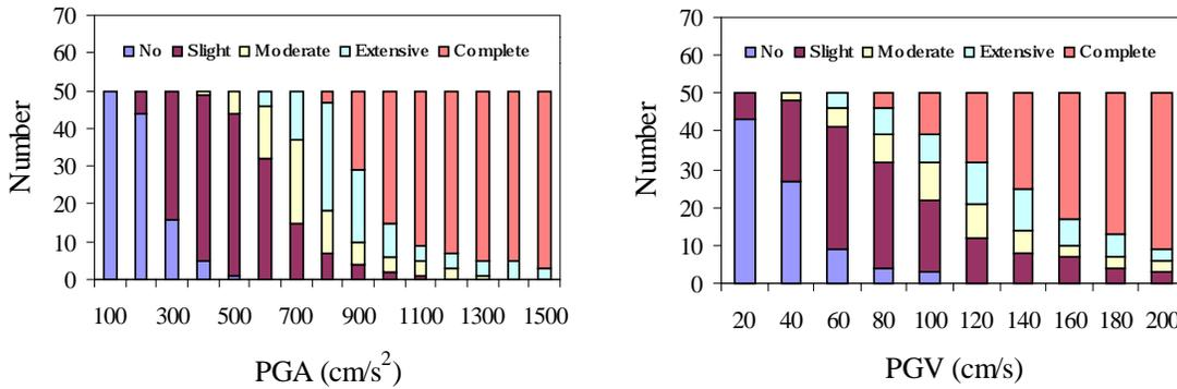
**Figure 1. Number of occurrence of each damage rank in different excitation levels.**
