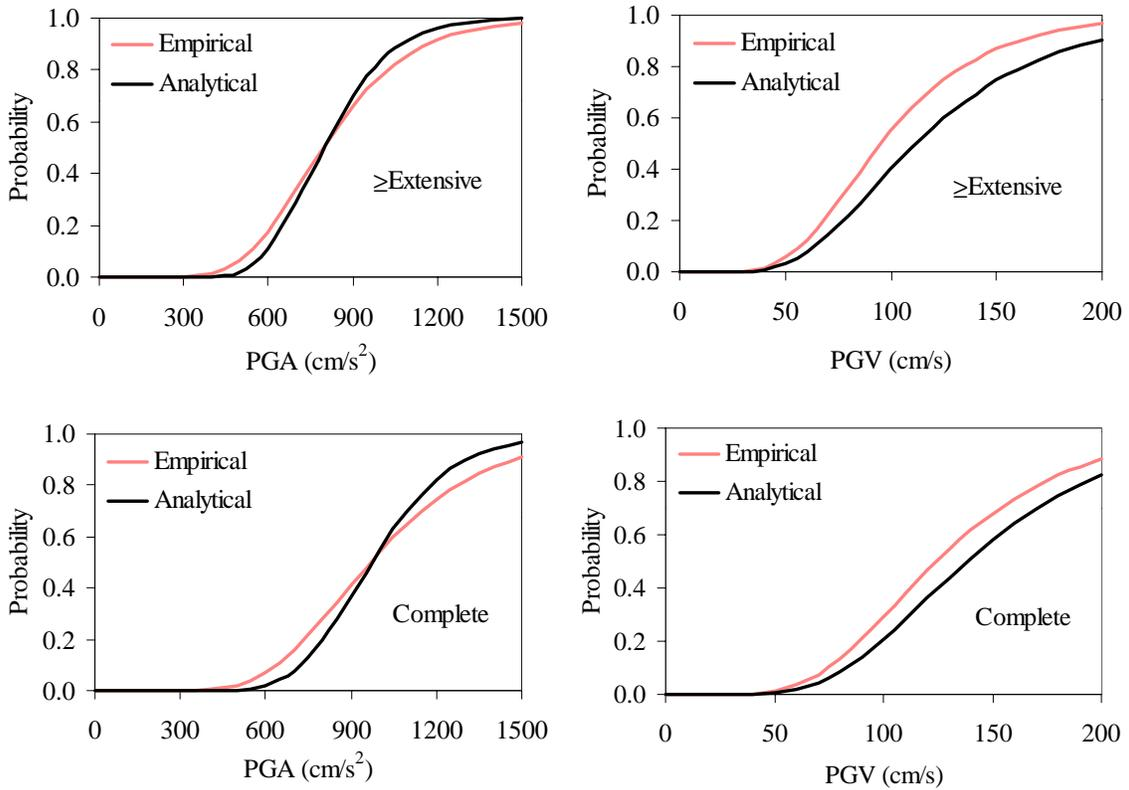
**Figure 3. Fragility curves for RC bridge piers with respect to both PGA and PGV from the records of the Kobe earthquake.**
