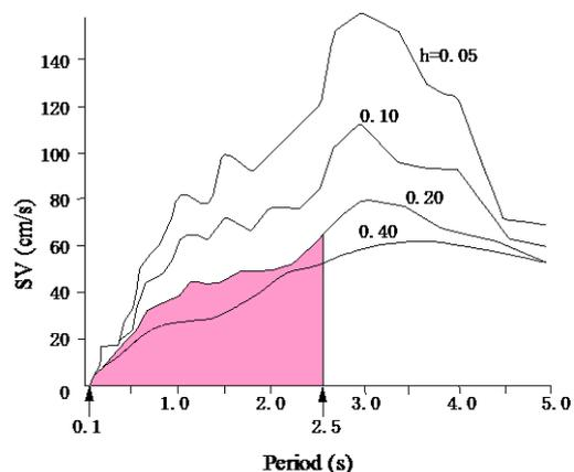
Figure 1. Definition of Spectrum Intensity: SI
