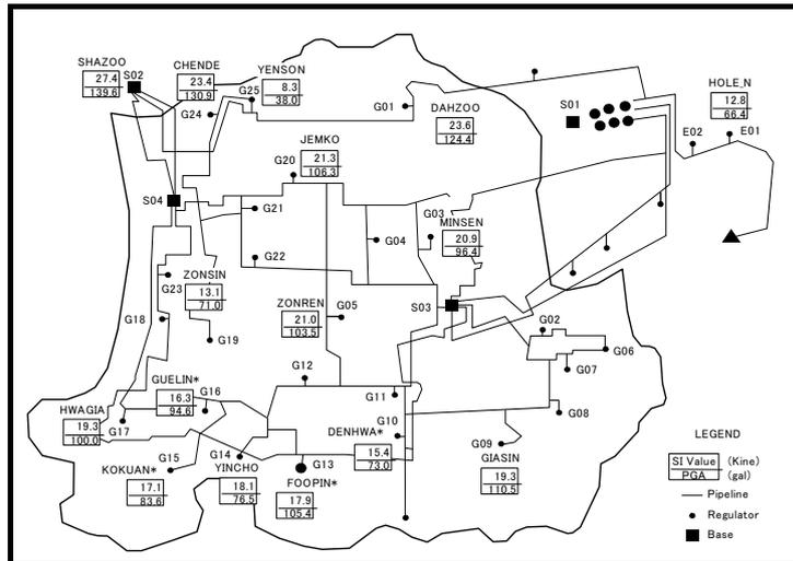
Figure 9. Distribution of SI and PGA in Taipei Observed by New SI Sensors in the 1999 Chi-Chi Earthquake
