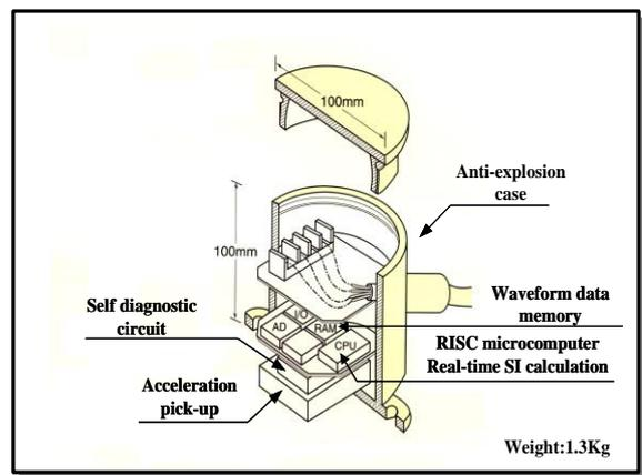
Figure 5. New SI Sensor
