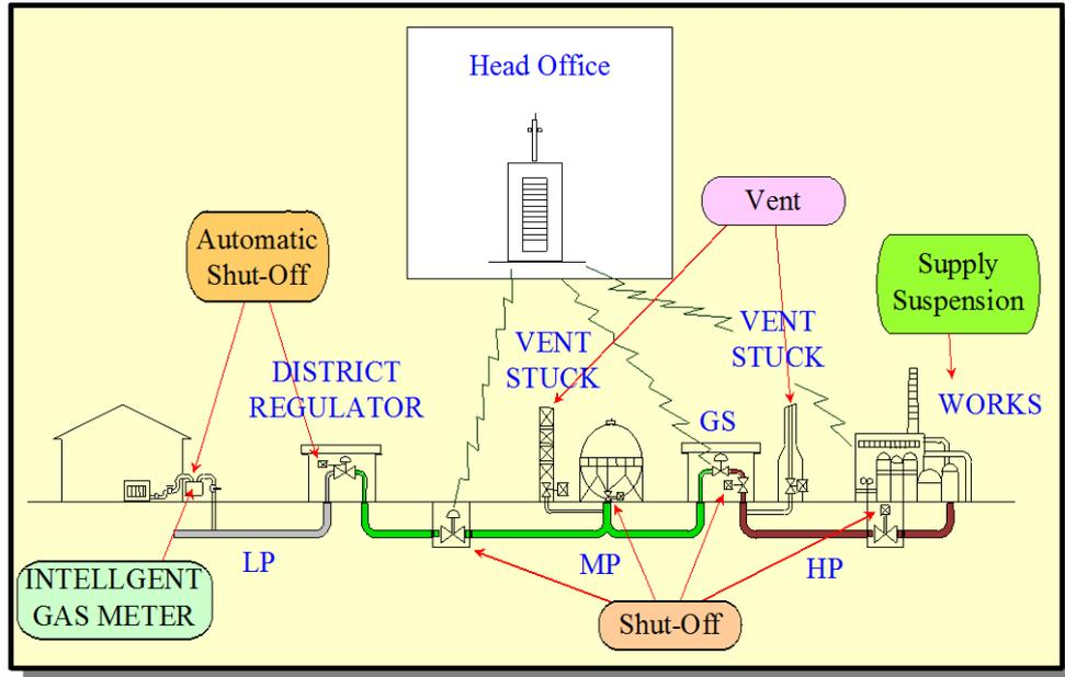
Figure 2. Emergency Shutoff Systems of Natural Gas Network of Tokyo Gas Co., Ltd.
