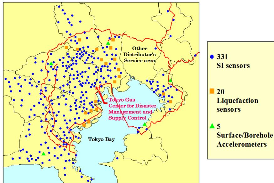
Figure 4. Seismic Monitoring Sensors of SIGNAL
