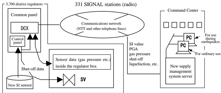
Figure 7. System Configuration of SUPREME
